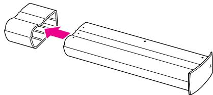
**Warning:** If you remove the battery, always place the plastic end cap over the battery terminals.
