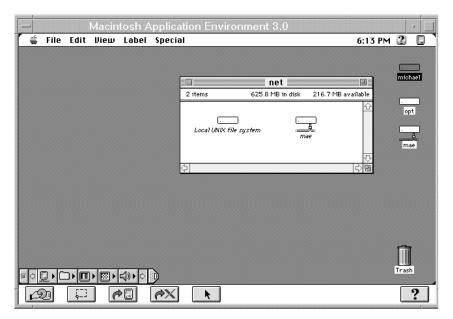
Note that the net folder contains the alias to the mae volume shown as an icon on the desktop. Double-clicking either the alias or the volume icon opens a window for the mae volume. No change has been made from the perspective of the UNIX file system. Listing the contents of the mae directory in UNIX shows the same contents as the open MAE window.
