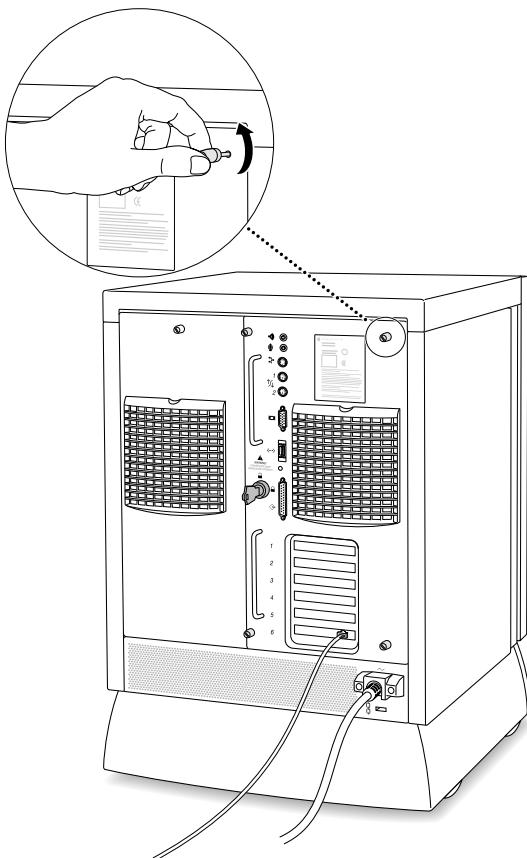
**5 Grasping the logic module by its handles, pull the module out as far as it will go.**
