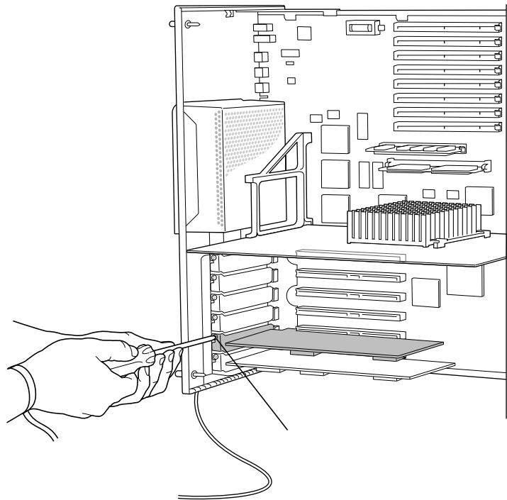
Once the card has been installed, push the logic module back in, tighten the thumb screws, turn the key to Lock, and reattach all cables. Do not turn on the computer until you have connected the card to the network.
