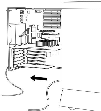
**6 Remove the cover plate from the expansion slot you want to use.**
