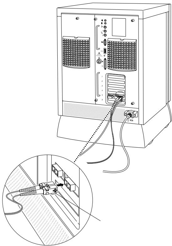
**IMPORTANT** Do not connect the Network Server to the next node on the network without consulting with your network administrator. Where and how you should connect, and how the rest of the network will be affected by adding a node, depends on your particular network.
