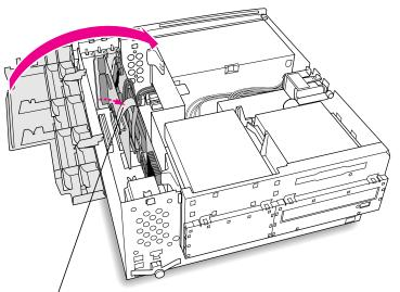
Bend the peripheral flex cable over as you close the expansion slot cover.
