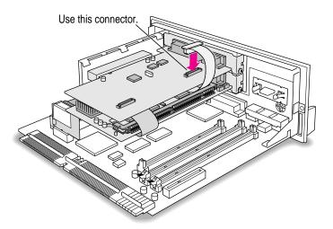
14 Push the peripheral flex cable down.
