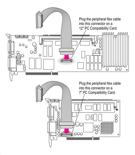
10 If you removed the PC Compatibility Card to attach the peripheral flex cable, then reinsert it now.
