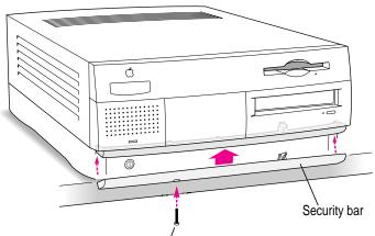
Install the screw in the hole on the underside of the security bar.
