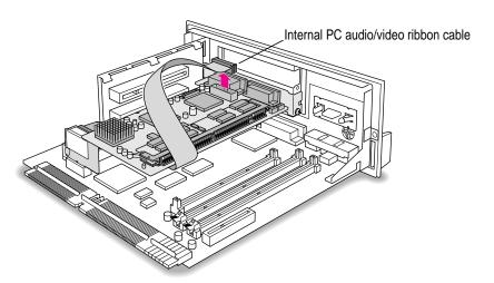
9 Attach the peripheral flex cable as shown.
