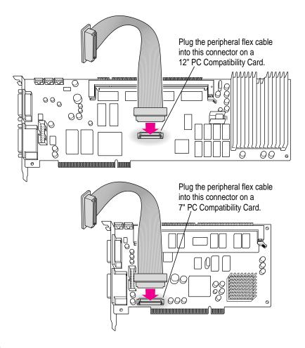
9 Insert the PC Compatibility Card into the second slot.
