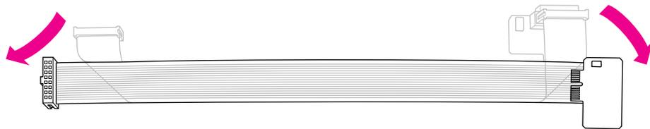
**2 Remove the rubber block from the large end of the internal PC audio/video assembly.**
