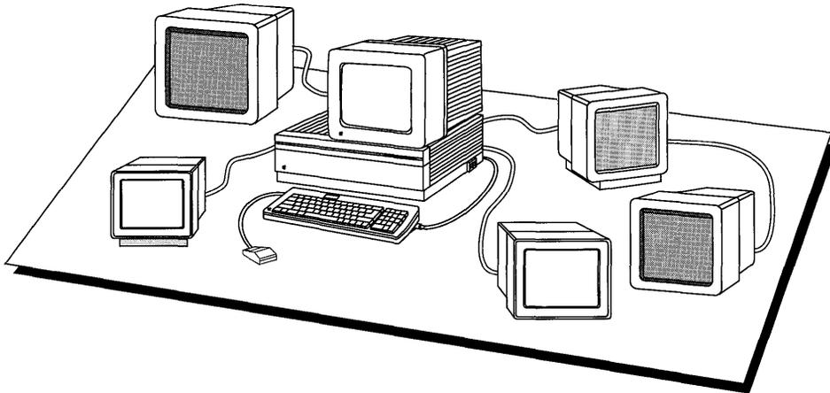
X11 is not designed for, nor does it support the use of, an ASCII terminal connected to a serial port. Rather, each monitor must be a high-resolution monitor connected to its own NuBus video card or to a built-in video port.
