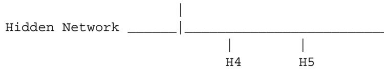
Proxy ARP technique (the ARP hack) allows one network address to be shared between two physical nets. Gateway G answers ARP requests on each network for hosts on the other network, giving its hardware address and then routing datagrams correctly when they arrive. In essence, G lies about IP-to-physical address bindings.
