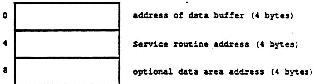
**Figure 4. ADBOp Parameter Block**
