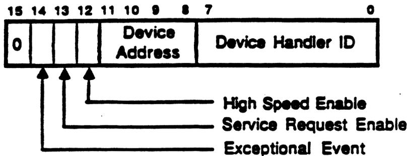
Figure 2. Layout of ADB Device Register 3.
