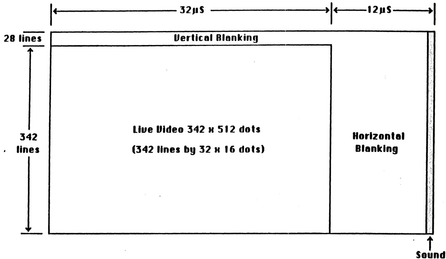
**Live video:** while the display is actively tracing a horizontal line of dots on the screen, video accesses to RAM (two words of data are read in each video access) alternate with three 68000 accesses.
