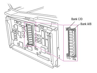
The DRAM SIMM installed in either of the SIMM slots must
