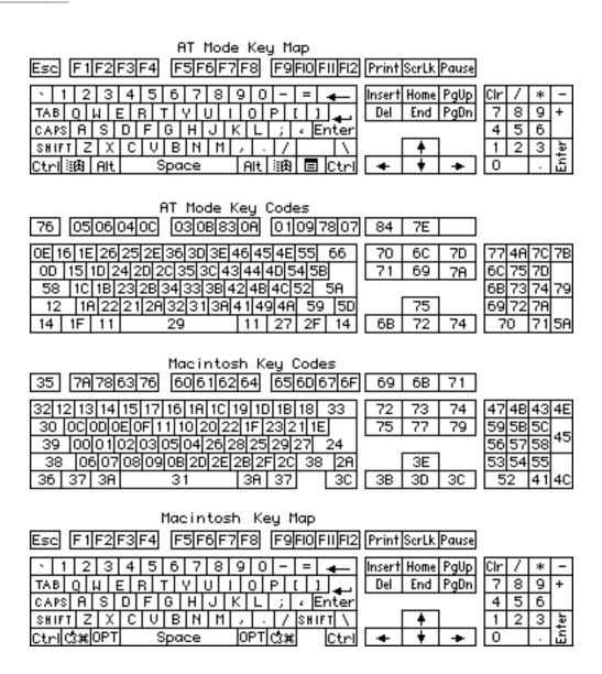
The AT keyboard to Macintosh keyboard key maps and key codes for the ID=3 AT key code translation ADB handler are shown in Figure 3-4.
