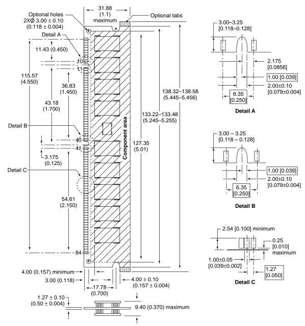
Note: dimensions are in millimeters (inches)
