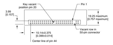
Note: Dimensions are in millimeters [inches]
