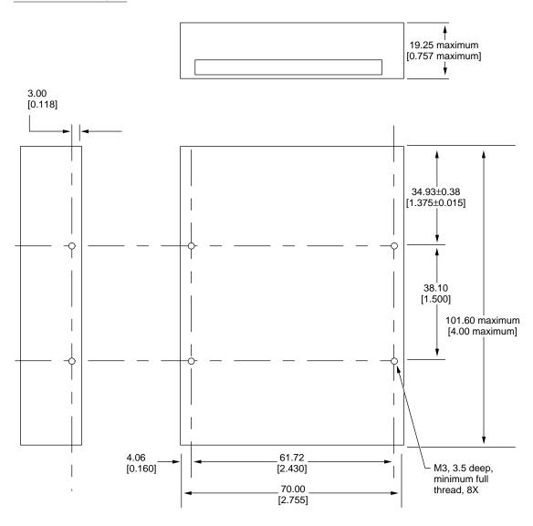
Note: Dimensions are in millimeters [inches].
