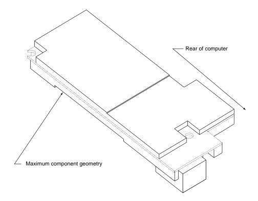
Figure 4-9 Maximum component heights on the top of the PCI expansion card
