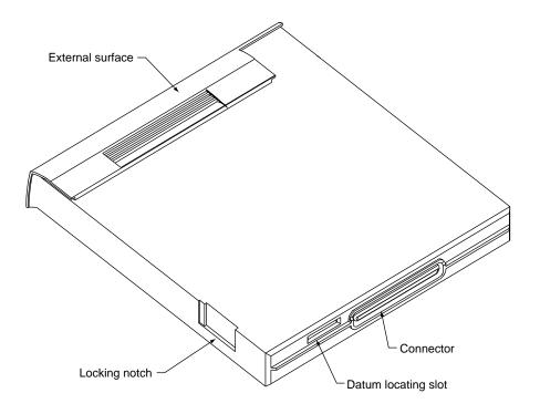
Figure 4-17 Location of expansion bay connector and datum slot
