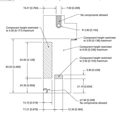
Note: Dimensions are in millimeters [inches].
