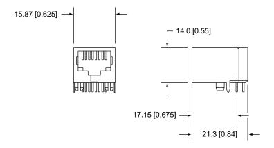
Note: Dimensions are in millimeters [inches].
