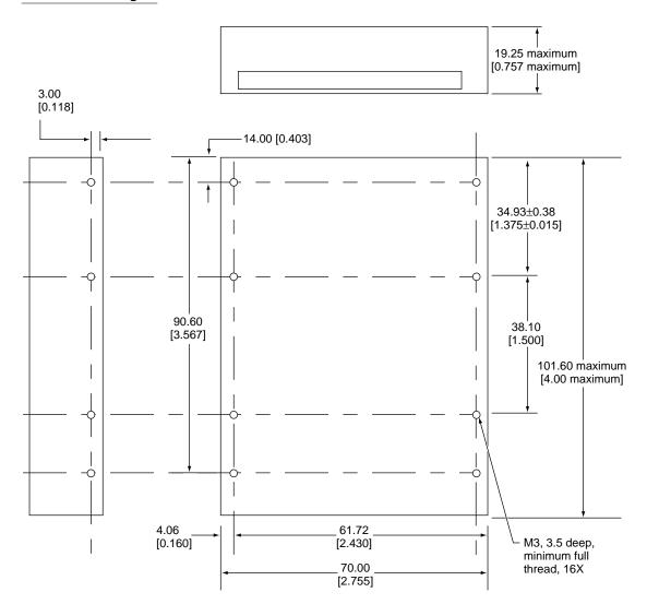
Note: Dimensions are in millimeters [inches].
