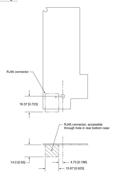
Note: Dimensions are in millimeters [inches].
