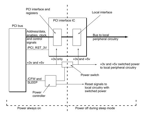
Depending on the power requirements of the devices on the expansion card, it may be necessary to provide low-power operation of the PCI interface IC. The circuit in Figure 4-13 is similar to the one in Figure 4-12, except it also switches the power to the PCI interface IC.
