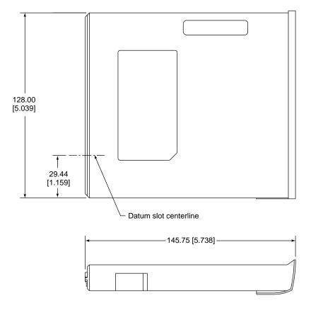
Note: Dimensions are in millimeters [inches].
