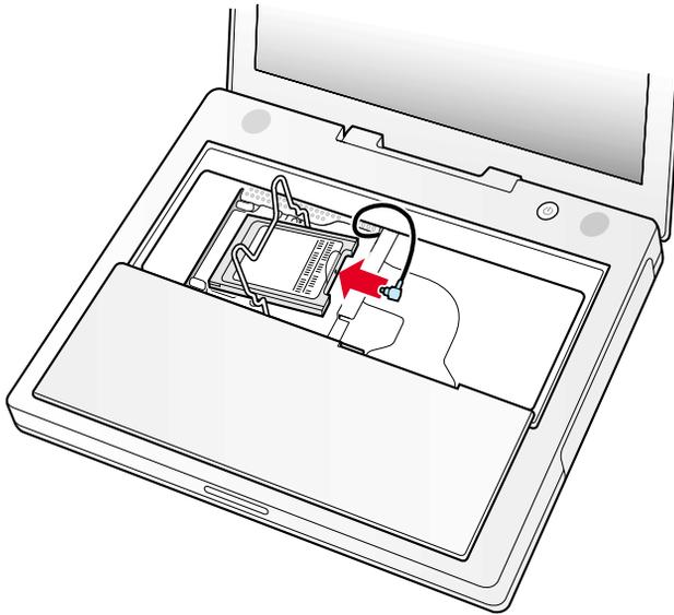
**Figure 4-2** The RAM shield plate
