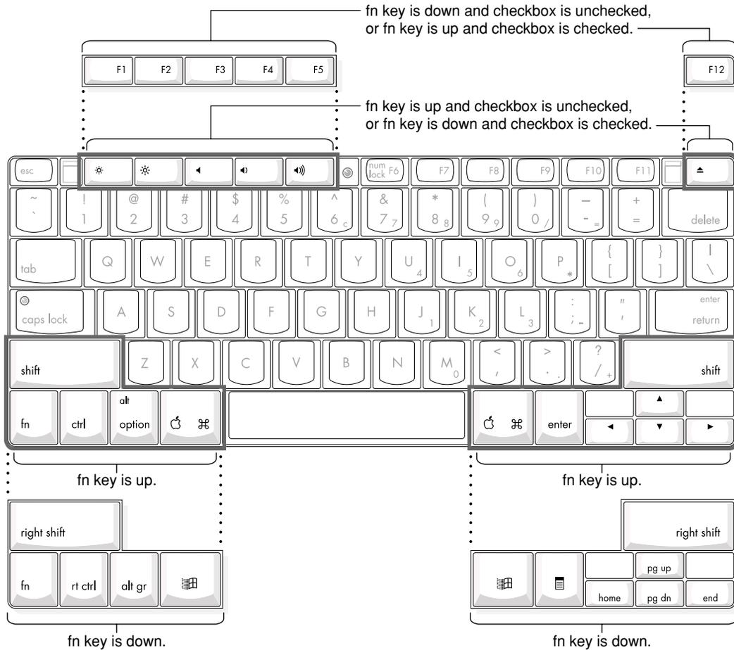
**Figure 3-9** Embedded numeric keypad operation
