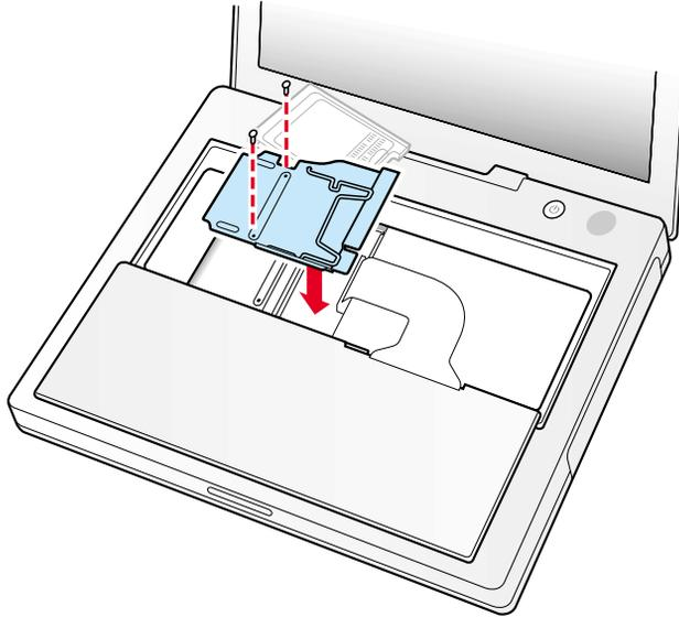
Once the RAM expansion module has been installed in the slot, the user must close up the computer by performing these steps in reverse order. Be careful to replace the shield plate properly so that the LAN card will fit.
