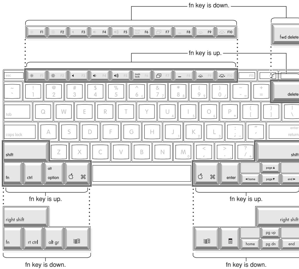
**Figure 3-8** Embedded numeric keypad operation
