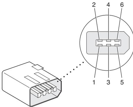
**Table 3-2** Pin assignments on the FireWire 400 connector
