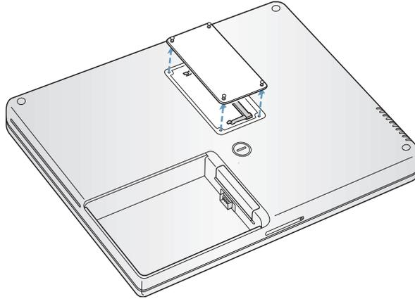
6. If a memory card is installed, release it by spreading apart the tabs in the expansion slot from the notches in the card. Allow the card to pop up slightly, and pull it out of the slot.
