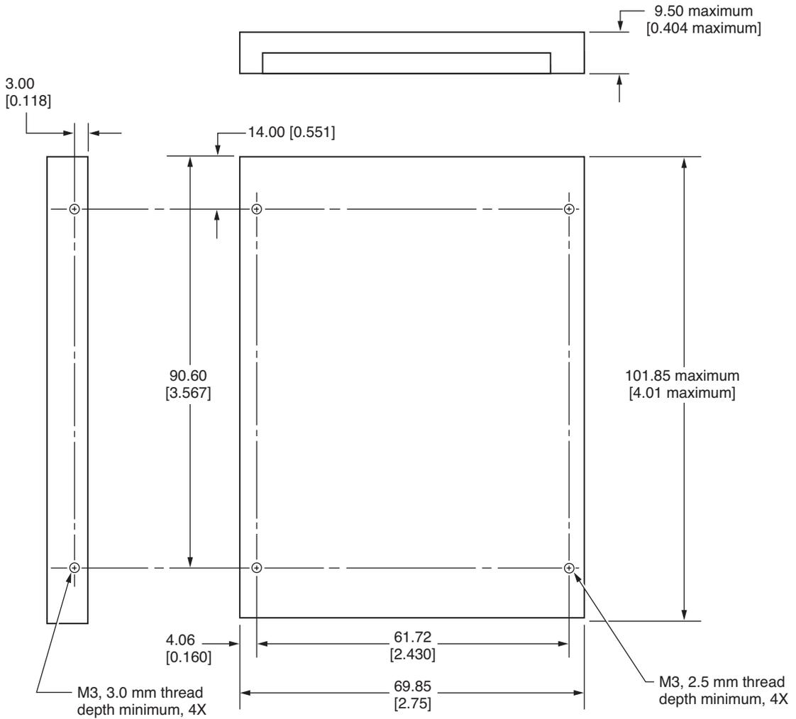
Note: Dimensions are in millimeters [inches].
