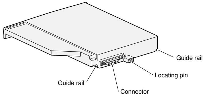
**Figure 4-3** Front view of a small expansion bay module
