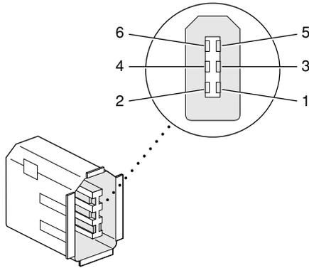
**Table 3-2** Pin assignments on the FireWire connector
