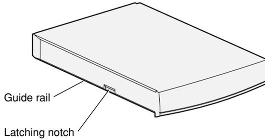
**Figure 4-4** Back view of a small expansion bay module
