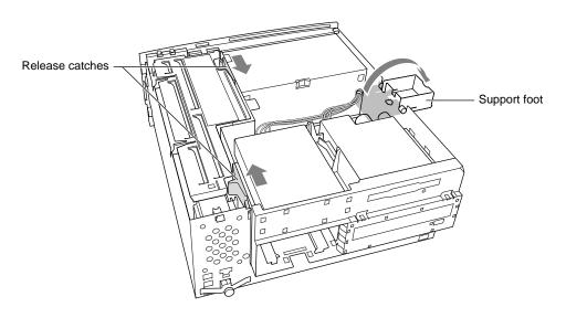
Figure 1-4 Top chassis in open position
