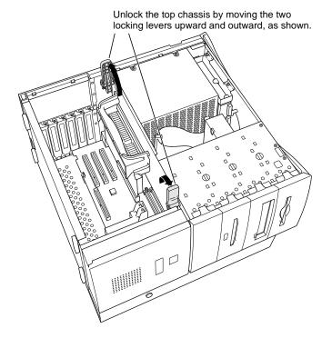
Figure 1-10 Lifting the top chassis
