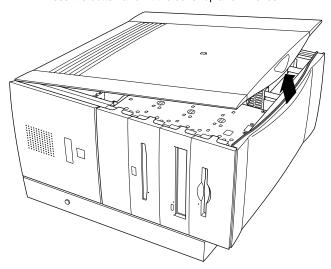
With the side panel out of the way, the user has access to the components at the bottom of the computer: PCI expansion slots, the DAV connector, and the space for internal RAID storage devices.
