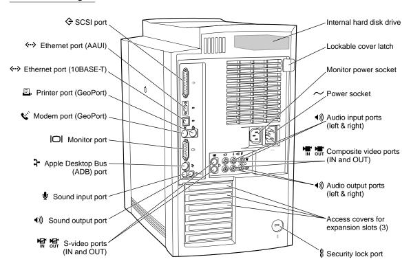
Figure 1-5 Front view of the Power Macintosh 9600
