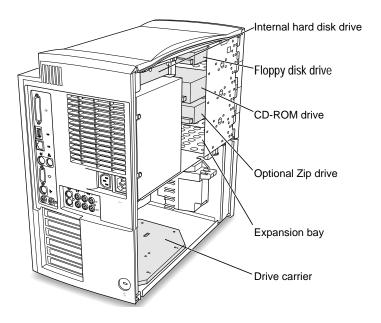
The floppy disk drive can be replaced with a 3.5-inch SCSI hard disk drive up to 1 inch high. The CD-ROM drive and the Zip drive can be replaced with 5.25-inch or smaller SCSI devices up to 1.625 inches high.
