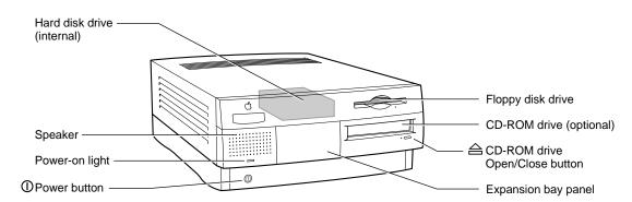
Figure 1-1 Front view of the Power Macintosh 7200 computer
