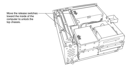
Figure 1-5 shows the top chassis in the open position.
