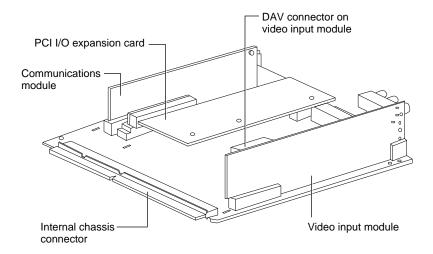
Figure 4-3 shows the orientation of the DAV connector on the video input module.
