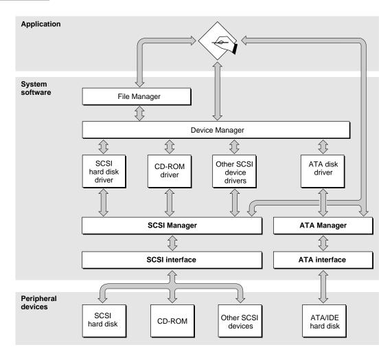
At the system level, the ATA disk driver and ATA Manager work in the same way that the SCSI Manager and associated SCSI device drivers work. The ATA disk driver provides drive partition, data management, and error-handling services for the Macintosh Operating System as well as support for determining device capacity and controlling device-specific features. The ATA Manager provides an interface to the ATA disk drive for the ATA disk driver.
