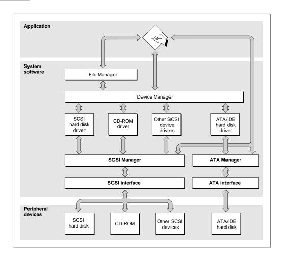
At the system level, the IDE device driver and ATA Manager work in the same way as the SCSI Manager and the associated SCSI device drivers. The IDE hard disk device driver provides drive partition, data management, and error-handling services for the Mac OS. It also determines device capacity and controls device-specific features. The ATA Manager provides the IDE device driver with an interface to the IDE hard disk drive.
