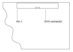
The DVA connector accepts YUV video and analog sound from the expansion card but does not itself generate YUV video output or audio output signals.
