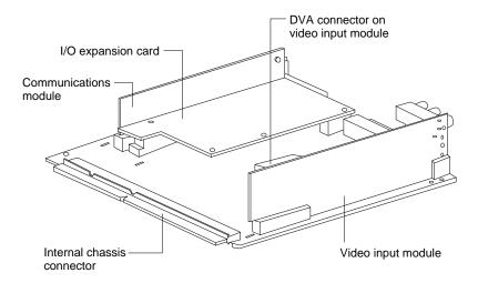
Figure 4-4 shows the orientation of the DVA connector on the video input module.
