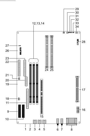
Table 3-1 lists the locations and types of connectors on the Power Macintosh 4400 logic board. Refer to the connector numbers in Figure 3-1 to determine the location of each connector on the logic board.
