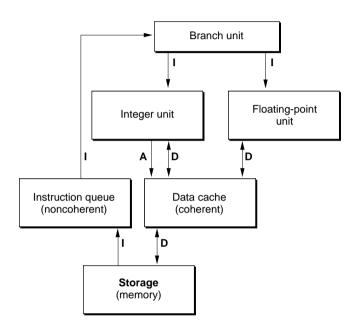
The memory storage shown at the bottom of Figure A-1—normally, the computer's DRAM—contains the program instructions to be executed and the data to be fetched, processed, and returned. The parts of the PowerPC microprocessor that execute the instructions and process the data are discussed in the next sections.
