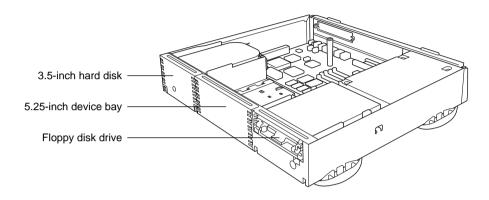
The location of the built-in CD-ROM drive in the Power Macintosh 7100/66 and 7100/66AV is shown in Figure 3-4.
