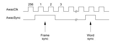
The AwacSync synchronization signals for each subframe are shown in Figure 3-14.
