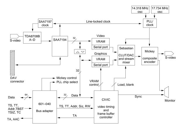
The video and graphics I/O system shown in Figure 3-10 is built around two banks of 80-ns VRAM with a total capacity of 2 MB. The CIVIC chip manages this VRAM and provides timing and interrupt signals. Applications can use the VRAM in two ways:
