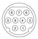
Either port can be independently programmed for asynchronous or synchronous communication formats up to 9600 baud, including AppleTalk and the full range of Apple GeoPort protocols. Through these ports, the computer can communicate with a variety of ISDN and other telephone transmission facilities by using external pods.
