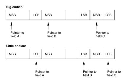
PowerPC processors and processors of the Motorola 68000 family use big-endian addressing; Intel processors use little-endian addressing. Different I/O chips, accessory card memories, and peripheral devices may use one addressing mode or the other, so data in versatile computing systems such as the Macintosh must often be accessed in either form.
