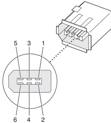
**Table 3-3** Signals on the 6-pin FireWire 400 connector
