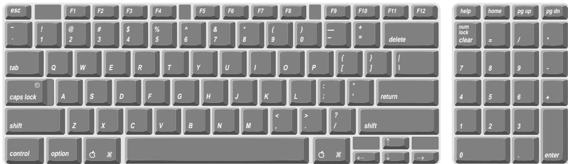
Power to the computer can be turned on using the power button on the Apple USB keyboard. A proprietary circuit allows the power control circuitry on the main logic board to detect a power-button press and turn on the power. The Apple USB keyboard can be used to turn on the power only if the keyboard is connected directly to the computer or is connected to an Apple Studio Display with a USB hub that is connected directly to the computer.
