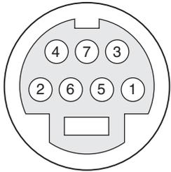
**Table 3-11** Pin assignments for the S-video output connector
