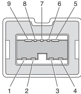
**Table 3-2** Signals on the 9-pin FireWire 800 connector
