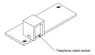
Figure 4-18 Top view of a simple DAA card
