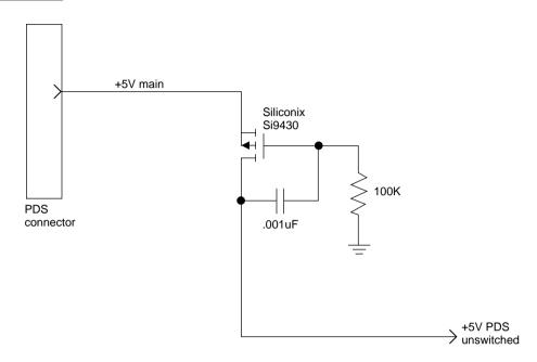
Figure 4-7 Recommended power control circuit
