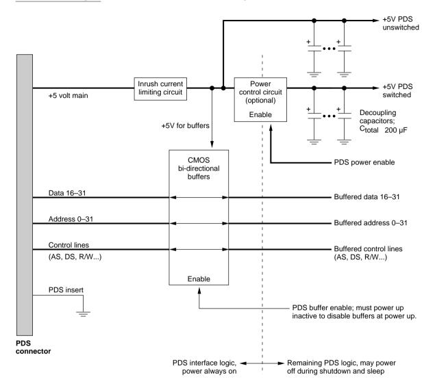
The bus interface controller on the PDS card should provide a register-controlled reset to the rest of the logic on the card. That arrangement makes it possible for software to reset the devices on the PDS card whenever it restores power to the card.
