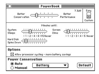
In custom mode, the PowerBook control panel lets the user set the time delays in minutes until the computer dims the display, goes into sleep mode, and goes into shutdown mode. The user can also select processor cycling, which slows down the processor and saves power.
