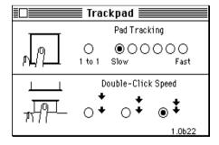
The Trackpad control panel allows the user to set the characteristics of the trackpad to match the way the user operates it. The user can set the scale and sensitivity of the trackpad and the time interval for a double click.
