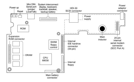
Figure 1-3 shows the locations of the supporting logic components on the bottom of the PowerBook 150 main logic board.
