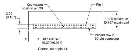
Note: Dimensions are in millimeters [inches].
