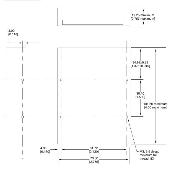
Note: Dimensions are in millimeters [inches].
