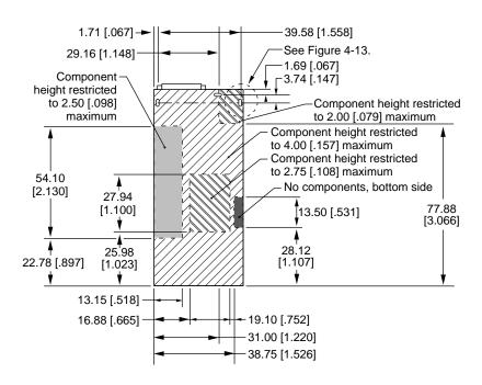
Note: Dimensions are in millimeters [inches].
