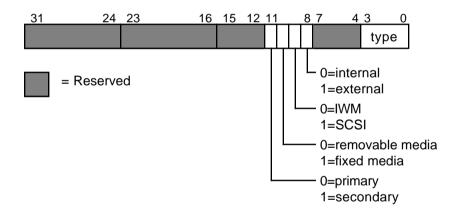
The attributes field occupies bits 8 to 11 and describes the location (internal/external, primary/secondary), drive interface (IWM/SCSI), and media type (fixed/removable).
