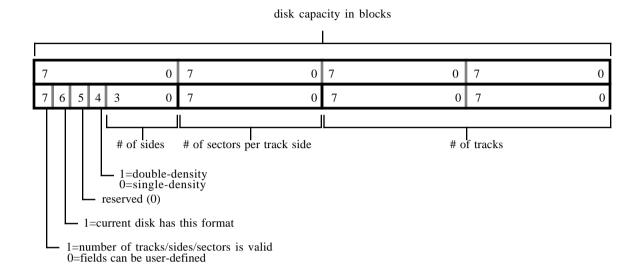
If a track, side, or sector field is zero when the *valid* bit is set to 1, the field is considered to be a "don't care" as far as describing the format of the disk. The formats supported by the driver are listed in Table 3–6.
