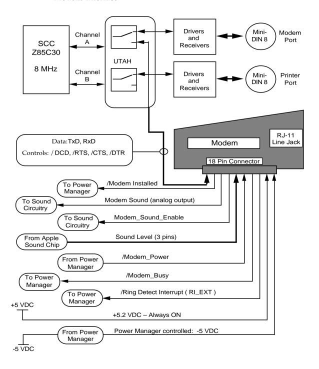
The data access between the Macintosh Portable CPU and the modem is an 18–pin dual inline socket connector on the modem card. The data is at TTL levels ( $V_{IL} = 0$  to 0.8 V;  $V_{IH} = 2.8$  to V+;  $I_{OL} = 1.6$  mA;  $I_{OH} = -25$   $\mu$ A).
