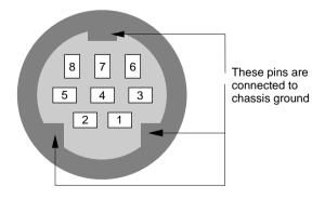
Table 14-6 Serial port connector signal assignments
