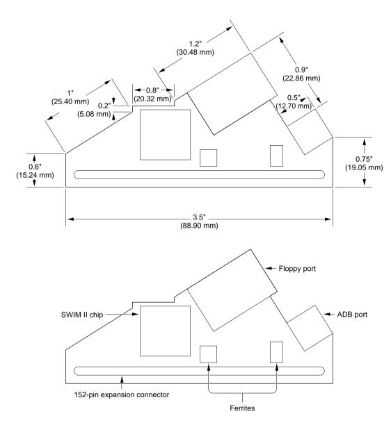
Figure 10-3 is a block diagram of the PowerBook Duo Floppy Adapter logic board functions. The logic board provides the facility to attach a floppy drive to the PowerBook Duo. It also routes the ADB signals from the 152-pin main expansion connector to the ADB connector.
