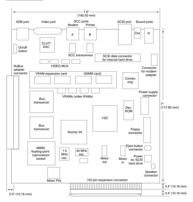
To reduce electromagnetic emissions, careful attention is given to the electrical design of the logic board. Parallel RC networks on connector signals reduce high-frequency noise. Using series termination for all long multiple-loaded signal paths reduces reflection.
