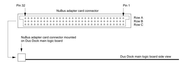
Figure 14-13 NuBus adapter card mounting configuration
