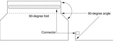
Figure 11-3 Macintosh Duo MiniDock logic board with dimensions
