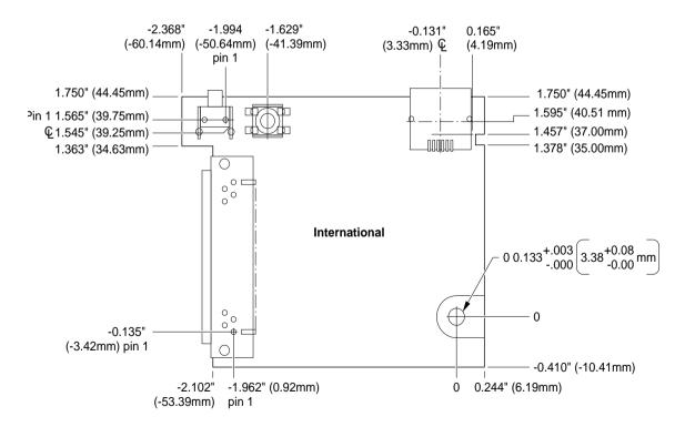
Figure 5-3 Modem card component height
