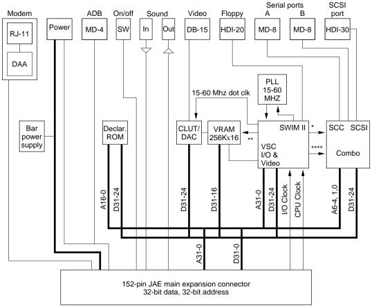
I/O Clock = 15.6672 Mhz CPU Clock = 33.3333 Mhz
