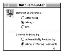
Using Remount Shared Disks, you can choose to implement the feature after sleep, after shutdown or sleep, or turn off the feature. When the PowerBook Duo goes into a sleep or shutdown state, the software determines which servers are mounted, and saves the
