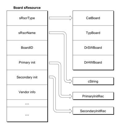
The PrimaryInit entry contains an offset to a PrimaryInit record. If the PrimaryInit record is not present, the computer assumes that the card initializes itself or does not require initialization. For the PowerBook declaration ROM, PrimaryInit contains interrupt handlers and video initialization code.
