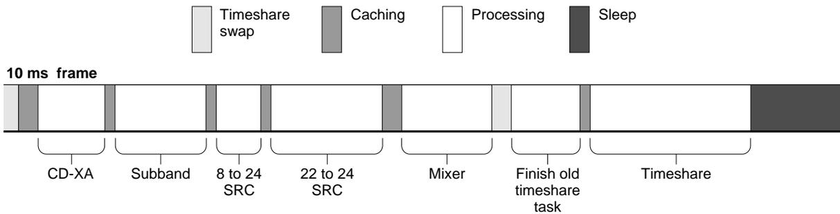
As Figure 3-12 shows, the five required real-time processing modules are run in sequence. The timeshare algorithm that was running when the frame started is reloaded and completed. One more timeshare algorithm is run, and since no more timeshare algorithms are active in this example, the DSP goes to sleep and waits for the next frame interrupt.
