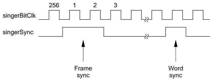
The `singerSync` synchronization signals for each subframe are shown in Figure 2-17.
