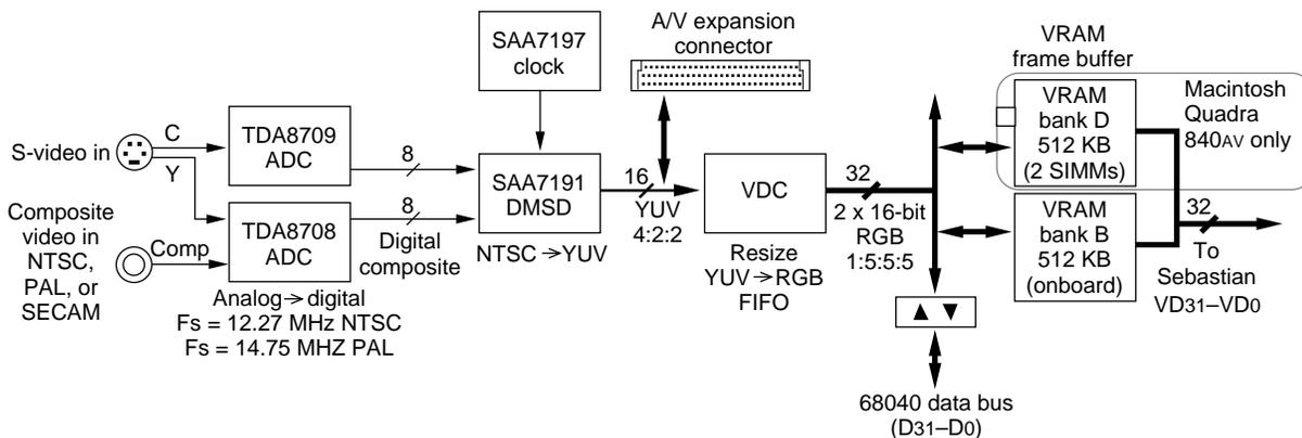
The input signal, which may be analog composite or S-video in NTSC, PAL, or SECAM format, enters through an external 7-pin mini-DIN socket. A cable adapter is provided to receive composite video from external devices that have RCA connectors. TDA8708 and TDA8709 video ADC chips digitize the composite video waveform, and the DMSD chip decodes the result into YUV format. This common digital video format, also known as YCrCb, is described in CCIR Recommended Standard 601-2.
