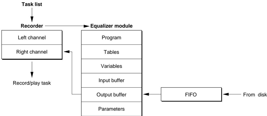
When the connection is made from the output buffer to the right channel buffer, the Clear flag is cleared, since this module is not the first to input to the right channel buffer. Likewise, the Save flag is cleared, since the right channel buffer already exists on-chip. Thus, any already existing signal in the buffer is directly summed into by the equalizer. This is a normal or *direct connection*.
