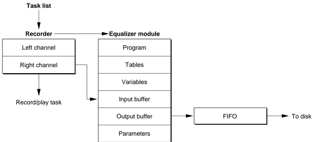
In this example, assume that the equalizer is monophonic. Its input buffer is a scalable AIAO buffer, and its output buffer is a scalable AIAO buffer. This means that the Load flag is set for the input buffer, and the Clear flag and Save flags are set for the output buffer. These buffers were created using the `NewScalableInputBuffer` and `NewScalablePRBOutputBuffer` macros.
