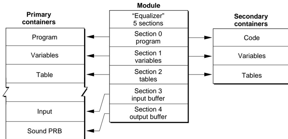
In the example, the code, variables, and table sections are loaded into the cache before the code section is executed. After execution completes, only the variables are saved back to local memory. It is important to recognize that the input and output buffers are not moved, but exist in the cache. This buffer mechanism is described in "Buffer Connections Between Modules" and "Buffer Connections Between Tasks," later in this chapter.
