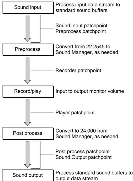
The sound input task takes the serial data stream from the DMA channel coming from the stereo A/D converter and converts it to DSP floating-point format. For 10 ms frames and 24 kHz sound, this takes the form of two 240-longword buffers. These buffers are established as ITBs by the DSP map structure associated with sound input.
