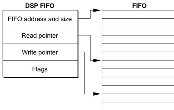
Each FIFO requires two separate blocks of memory: the `DSPFIFO` structure located in local memory and the FIFO itself located in either local memory or main memory. Usually, large FIFOs are placed in main memory by the client, to conserve the limited local memory space.
