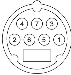
**Table 2-12** Video input connector pin assignments
