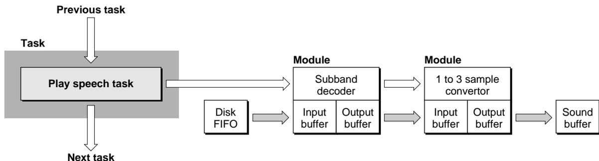
Notice that there are two types of connections in the diagram. First is the control flow, indicated with solid arrows. These are the connections that the DSP operating system follows to execute the real-time task list. The second type is the data flow connection, indicated by shaded arrows. In this example, data flows from the disk FIFO to the subband decoder module, from the decoder to the sample rate converter module, and from the converter module to the sound buffer.
