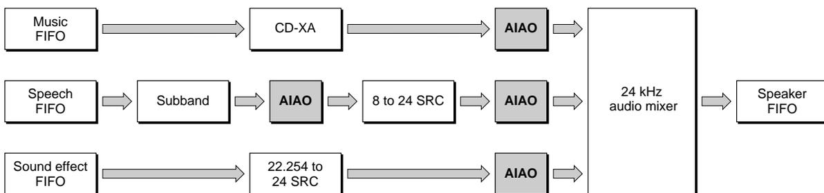
AIAO buffers are structured differently from FIFO buffers; they do not contain the header block found in the FIFO. They have a standard section structure and can be used in place, without being moved. It is these characteristics that make the AIAO buffer so efficient.
