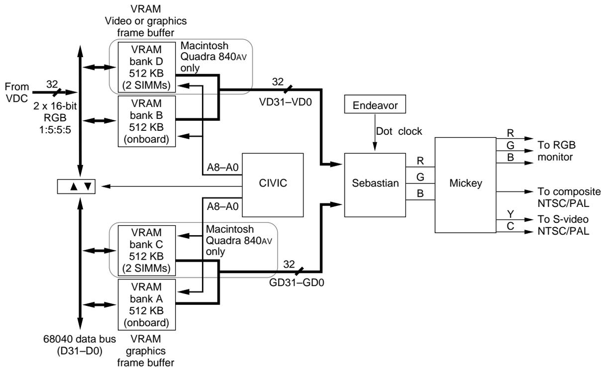
If the VRAM is configured as a single video frame buffer, it can all be used for graphics and the video input can be disabled. In this case, the CIVIC controls data access to VRAM from the following sources:
