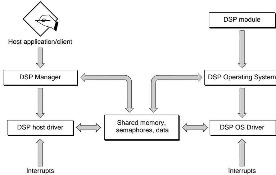
In most applications the DSP will need to run several different code modules or algorithms in sequence to process blocks of data. For example, five different DSP modules are required for a sound player to mix the following three channels of sound:
