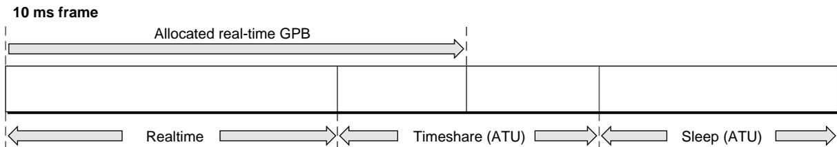
As shown in Figure 3-16, the ATT value is not necessarily the difference between the frame processing capacity and the GPB allocated to real-time tasks. It is often the case that real-time tasks are inactive, or not running at full processing bandwidth. This makes additional timeshare processing available.
