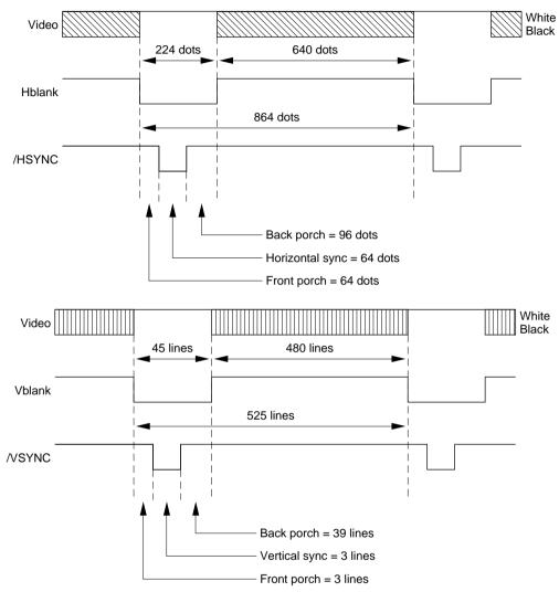
Dot clock = 30.2400 MHz Dot = 33.07 nS Full line =  $28.57 \mu s$ Line rate = 35.0 kHz Full frame = 15.0 mS Frame rate = 66.67 Hz
