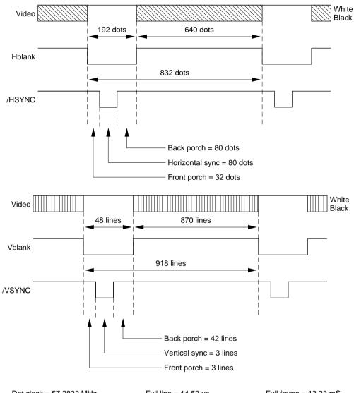
Dot clock = 57.2832 MHz Dot = 17.457 nS Full line = 14.52 µs Line rate = 68.850 kHz Full frame = 13.33 mS Frame rate = 75 Hz
