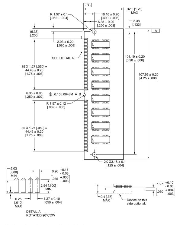
Note: Dimensions are in millimeters with inches in brackets.
