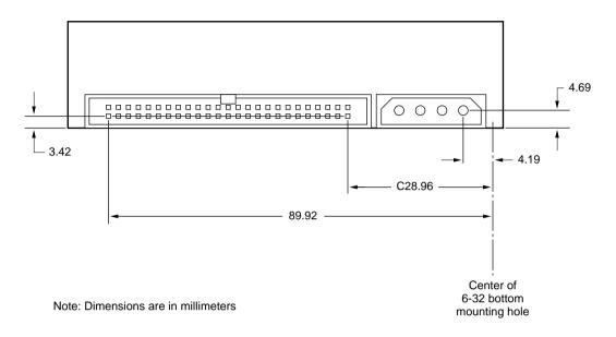
Figure 5-5 Dimensions of the CD-ROM drive
