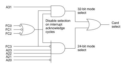
Figure 3-1 Generating the card select signal
