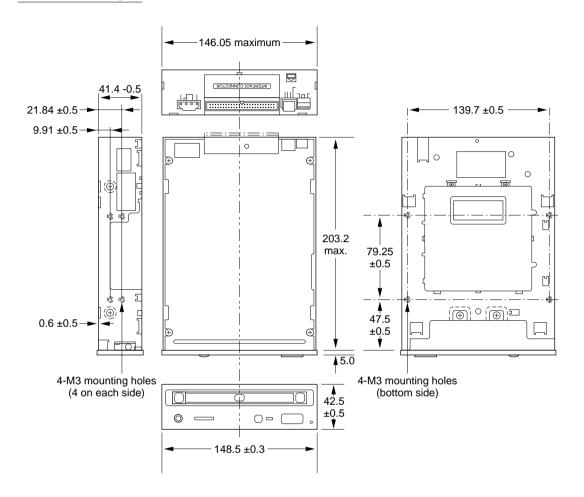
Figure 1-9 Mounting rail for 5.25-inch devices
