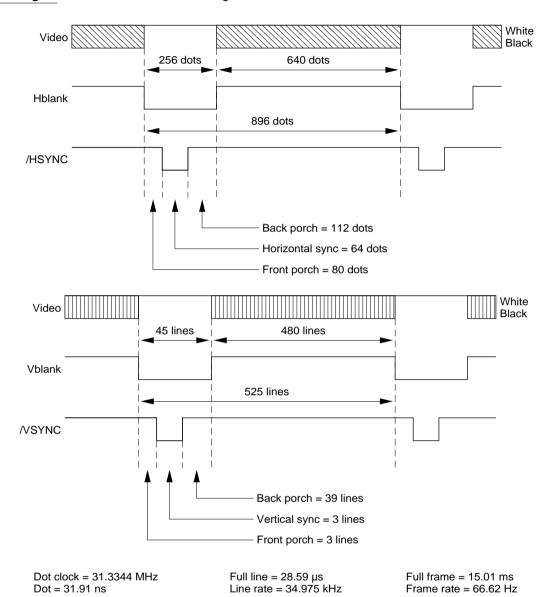
**Figure 1-4** 640 x 480 VGA timing
