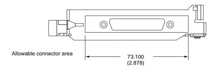
The 7-inch version of the NuBus card can be used in any Macintosh computer that has NuBus slots. Figure 3-5 shows how a 7-inch NuBus card aligns with a standard NuBus card.
