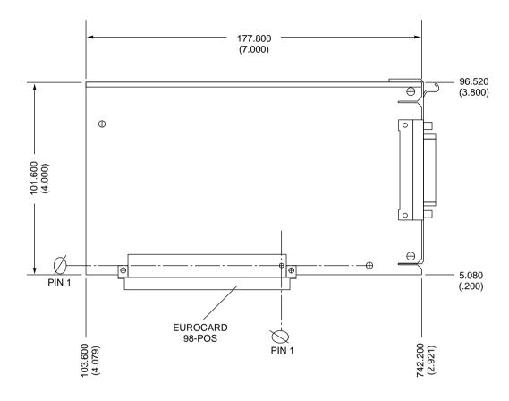
Note: Dimensions are in millimeters with inches in parentheses.
