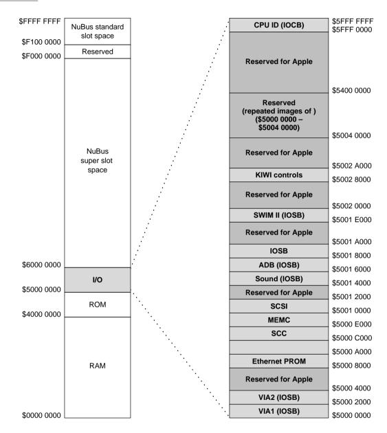
Figure 2-5 Addresses of expansion slots
