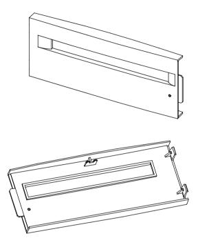
Foldout 1 is a design guide for the bezel used with the AppleCD 300i in the Macintosh Centris 610 computer.
