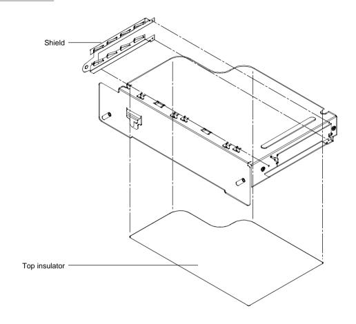
The folded 11 by 17-inch pages at the back of this note include design guides for the expansion bracket shown in Figure 3-2. Foldout 10 is a design guide for the shield bracket. Foldout 11 is a design guide for the insulator for the top of the adapter bracket. Foldout 12 is a design guide for the EMI shield for the adapter bracket.
