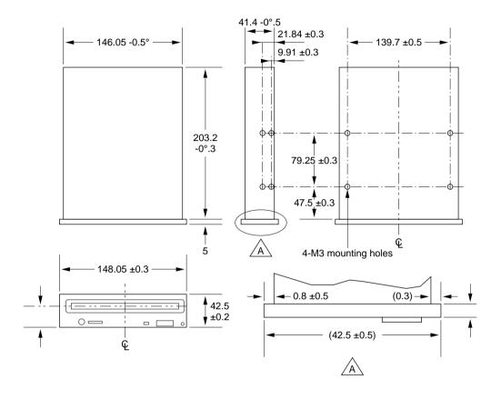
NOTE Dimensions are in millimeters.
