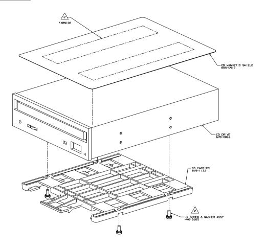
Foldout 2 is a design guide for the sled used for a 5.25-inch device in the Macintosh Centris 610 and Macintosh Quadra 800 computers.
