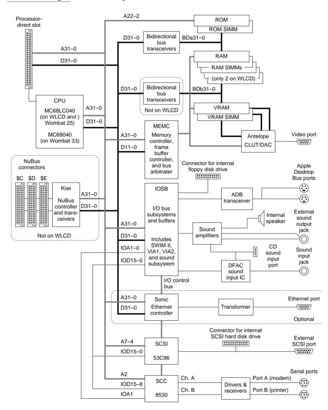
The MC68040 is different in many ways from the MC68020 and MC68030. For example, the MC68040's built-in FPU is not the same as the MC68881 FPU; similarly, the built-in MMU is not the same as the MC68851 MMU or the built-in MMU in the MC68030. Also, the instruction and data caches in the MC68040 use a new mode called CopyBack mode. For information about these differences and the way they are reflected in the new ROM software developed for the MC68040, see Chapter 4, "Software."
