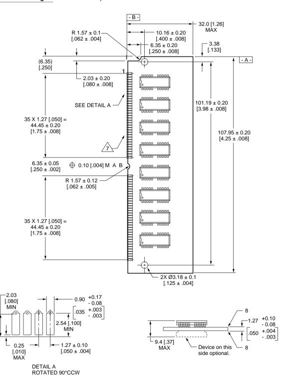
Note: Dimensions are in millimeters with inches in brackets.
