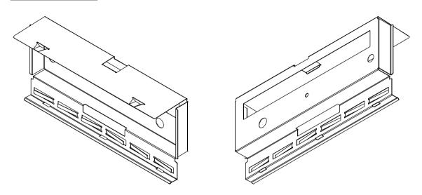
Foldout 3 is a design guide for the bezel shield used with the AppleCD 300i in the Macintosh Centris 610 computer.
