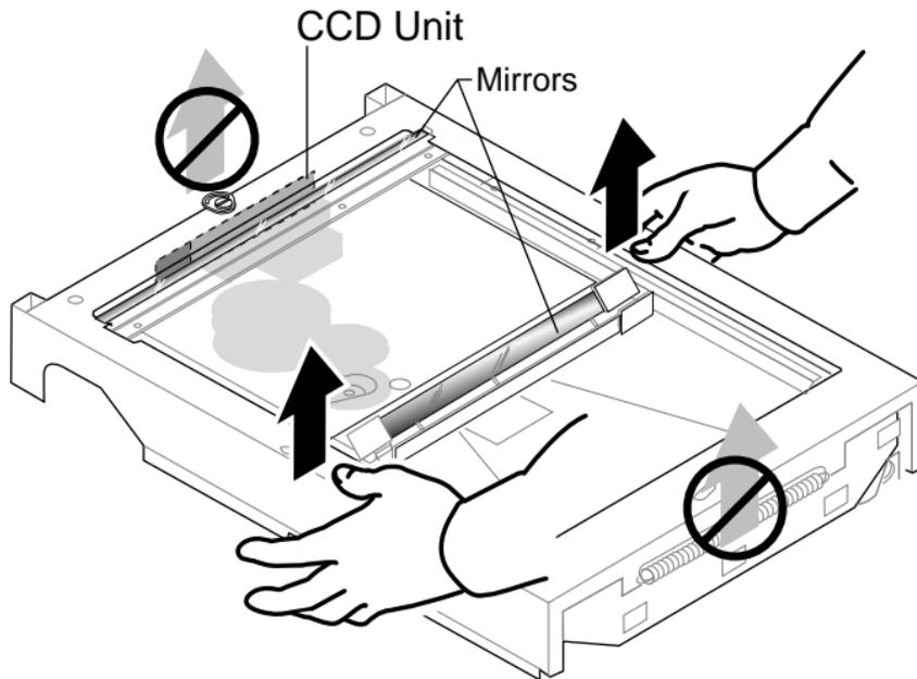
Hold or lift the optical assembly by the longer sides, never by the shorter sides.
