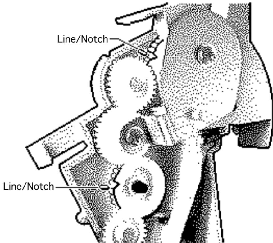
**Replacement Note:** Align the notch on the upper gear with the upper line on the cut sheet feeder. Align the notch on the lower gear with the lower line on the cut sheet feeder.
