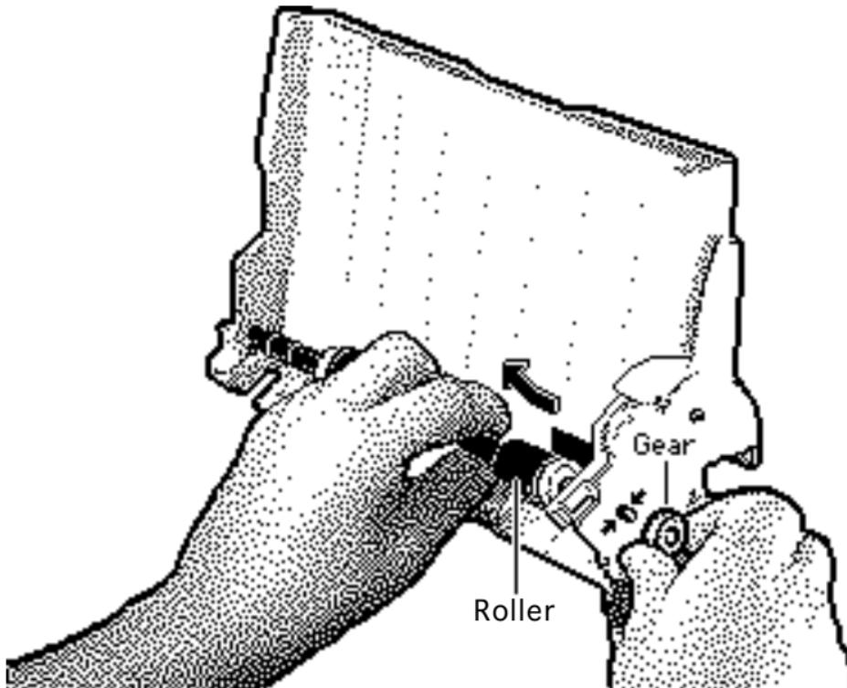
**Caution:** When the roller is removed, the feeder gear is loose. Remove the roller slowly so that the gear will not fly off.
