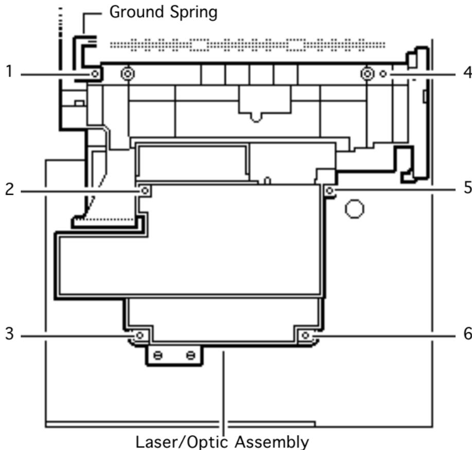
2 Remove the six screws that hold the laser/optic assembly to the printer base plate.
