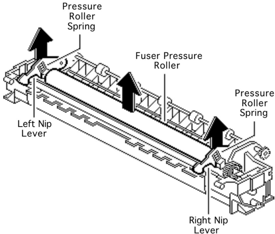
**Note:** The pressure roller springs and bearings easily fall off the nip levers.
