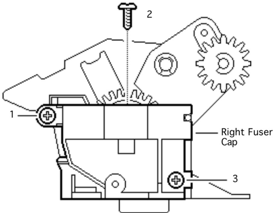
1 Remove the three screws that secure the right fuser side cap to the fuser assembly.
