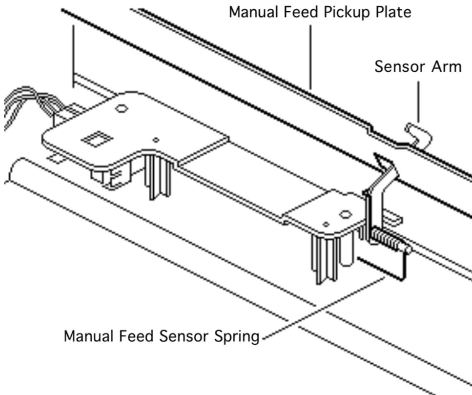
**Replacement Note:** Replace the sensor arm and spring as shown. The illustration shows the arm and sensor as they would look in a functional print-ready state.
