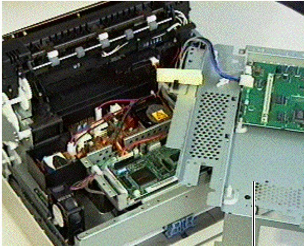
**Note:** Refer to "Test-Ready Configuration" in Basics for information regarding special handling of the I/O controller mount during troubleshooting. The photo on the left shows how the mount is positioned when the printer is in a test-ready state.
