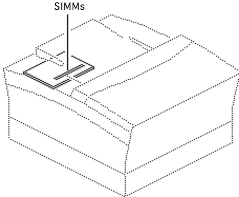
If you are upgrading the RAM in a LaserWriter Select 300 to 4 MB or more, perform the "Photograde Medallion" procedure in this chapter. The LaserWriter Select 300 requires a minimum of 4 MB of memory to print PhotoGrade images.
