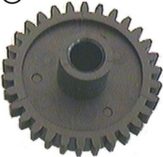
**Original 'Q' Gear w/damaged teeth**
