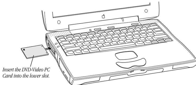
When inserting the card, you will feel some resistance. Continue to insert the card all the way into the lower PC Card slot. When completely inserted, only the end of the card (approximately 1/8 inch or 4 mm) will stick out of the PC Card slot.
