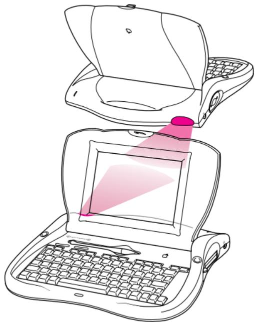
Infrared wireless transmission allows exchanging information with another eMate or Newton device, or connecting to a desktop computer. To do this, the infrared windows need to point directly at each other and should be less than one meter apart (closer in bright sunlight).
