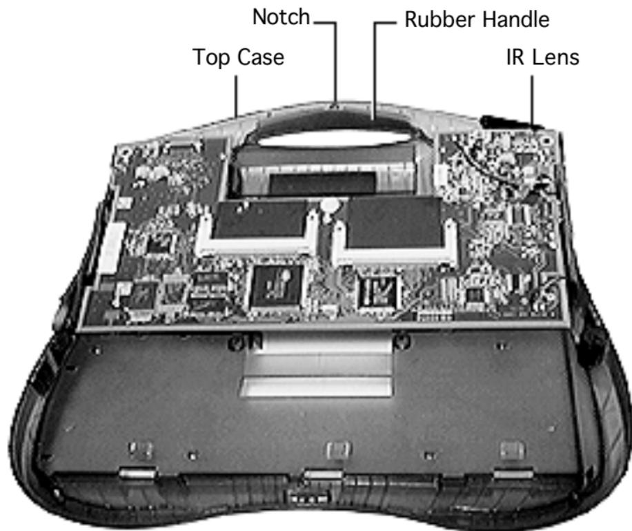
**Replacement Note:** Place the rubber handle on the top case so the notch faces up. Fit the IR lens into the top case. Hook the front of the bottom case first, then secure the bottom case onto the top case by pressing and rolling the sides.
