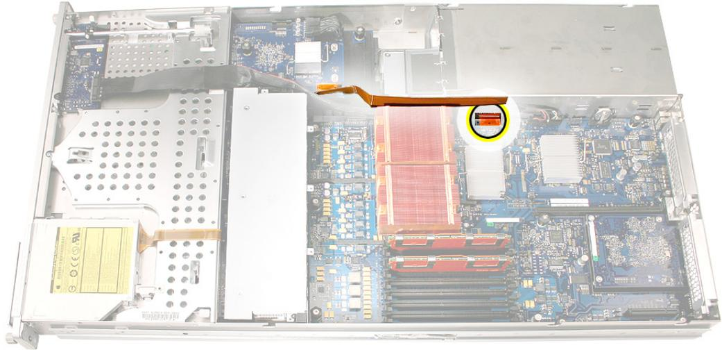
2. Disconnect the backplane-to-logic board cable from the drive interconnect backplane and remove the cable from the Xserve.
