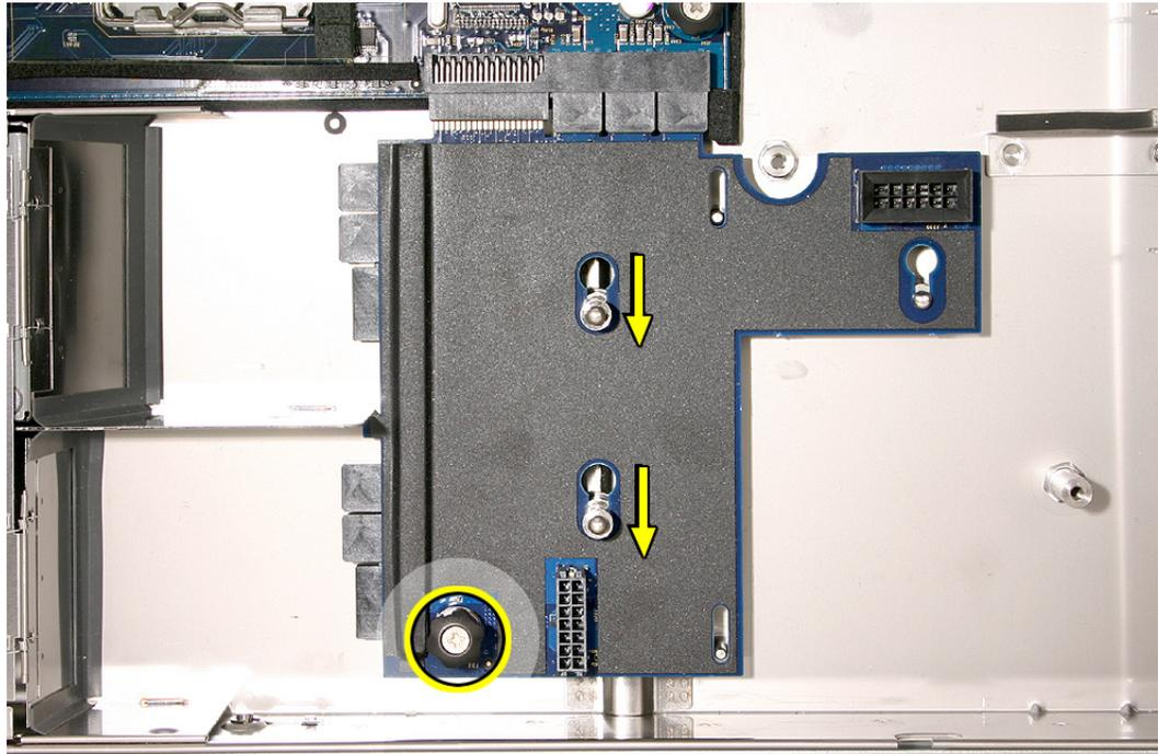
3. Lift up the board and remove it from the enclosure.
