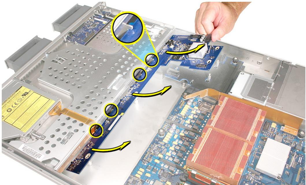
**Replacement Note:** When installing the backplane, lower the backplane into the enclosure at a slight angle (as shown), and carefully align the front edge of the backplane with the four backplane alignment slots in the enclosure. Be careful not to let any backplane components come into contact with the standoffs or the enclosure as you install the backplane.
