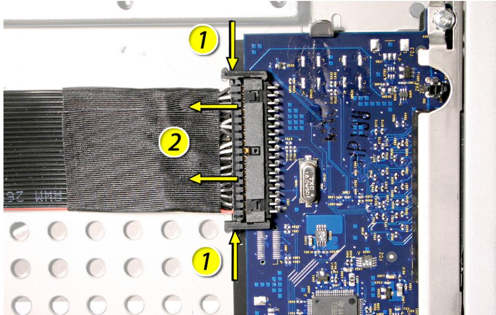
2. Disconnect the backplane-to-logic board I/O cable from the Xserve RAID Card.
