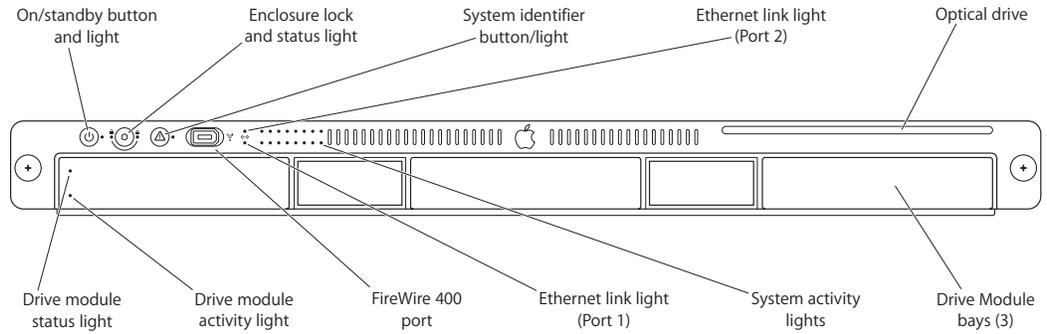
Note: The front bezel of the Xserve (Early 2008) model is identical to the Xserve (Late 2006) image above except the FireWire 400 port is replaced by a USB port, as shown below:
