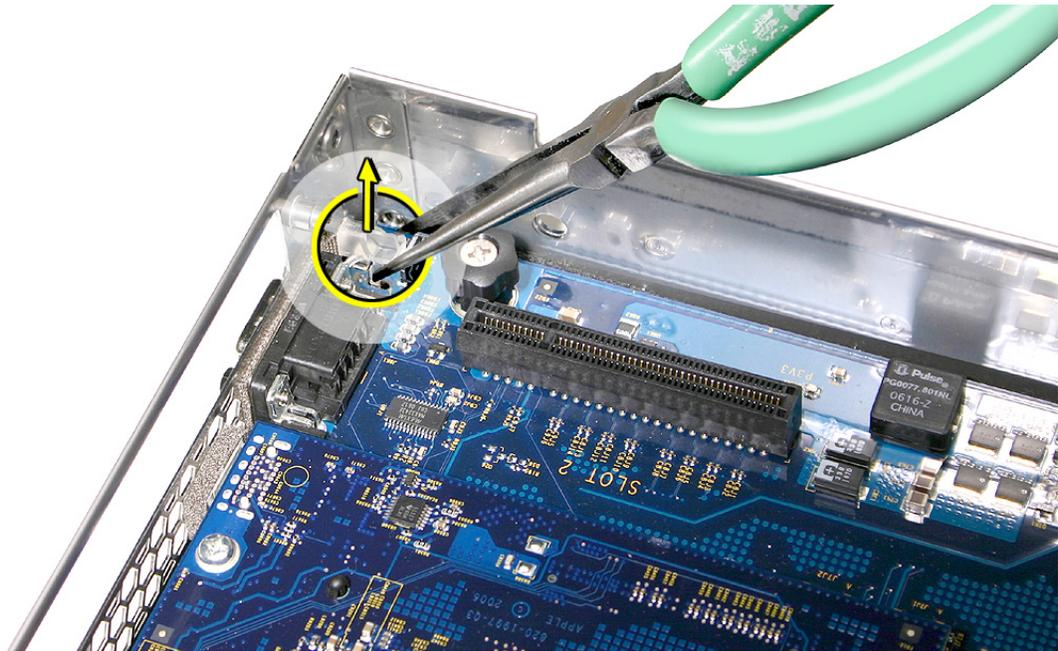
**Replacement Note:** When installing the rear ID button, take care not to bend or break the four small plastic prongs as you work the button back through the opening in the rear enclosure. Make sure all four prongs are properly seated in their respective holes in the logic board.
