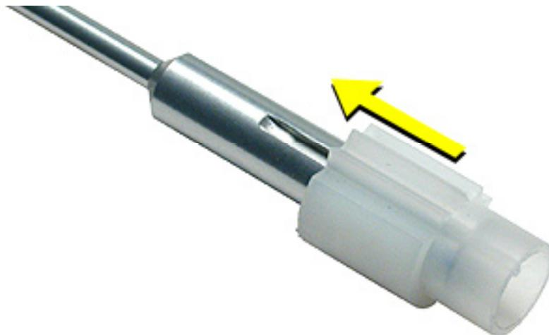
2. To install the locking rod, insert the key-hole end of the rod into the port on the front bezel.
