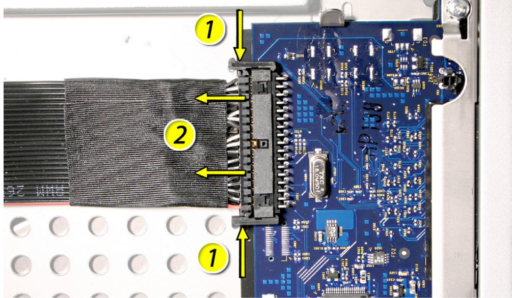
2. Disconnect the backplane-to-logic board I/O cable from the backplane.
