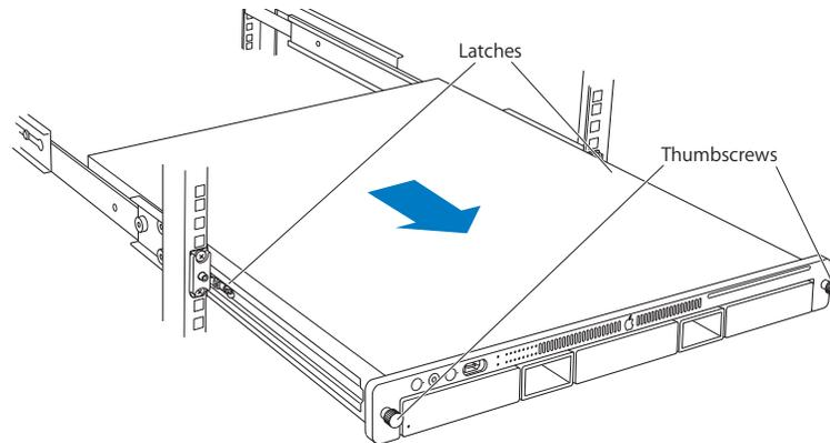
6. When the safety latches engage, grip the Xserve where it emerges from the rack, press down on the latch tabs with your thumbs, and slide the Xserve the rest of the way out of the rack rails. Set the Xserve on a flat surface.
