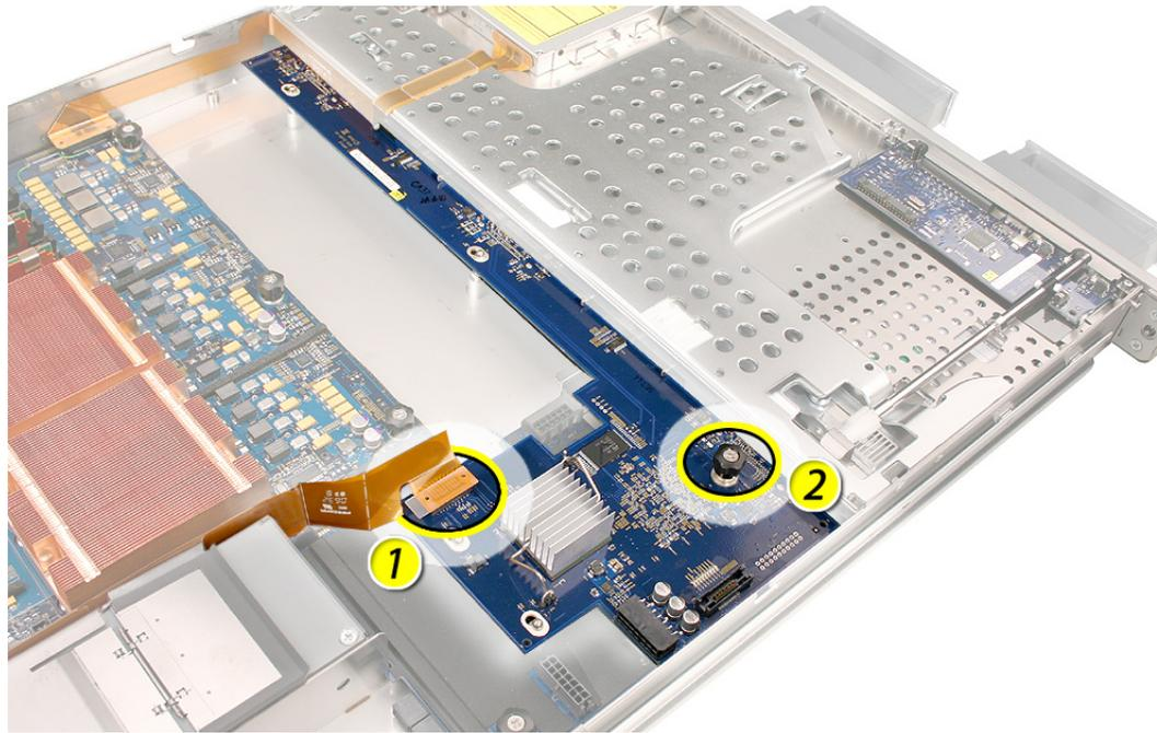
4. Shift the backplane to the left (towards the enclosure side), in the direction of the arrow shown, until it clears the four mushroom-shaped standoffs that hold the backplane in place.
