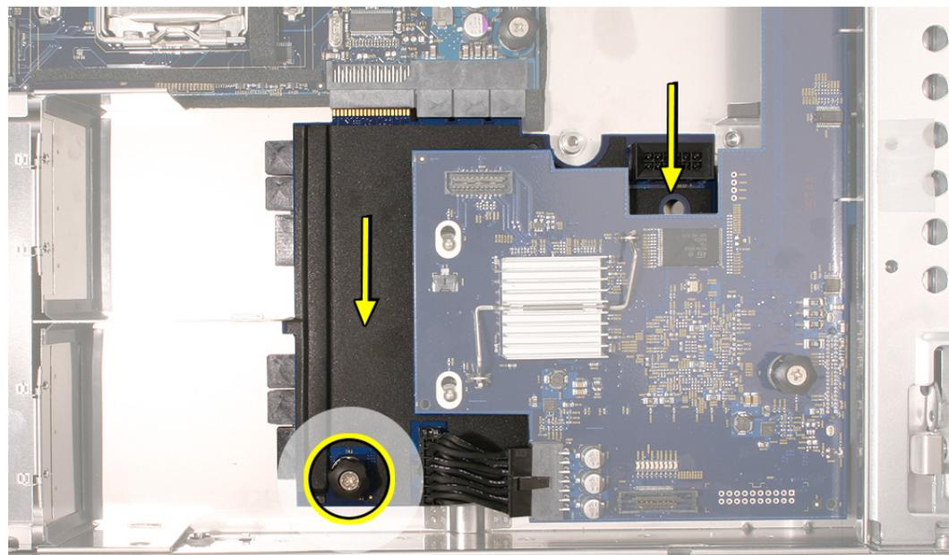
**Note:** Don't remove the power distribution board but make sure its edge connector is all the way out of the connector on the logic board.
