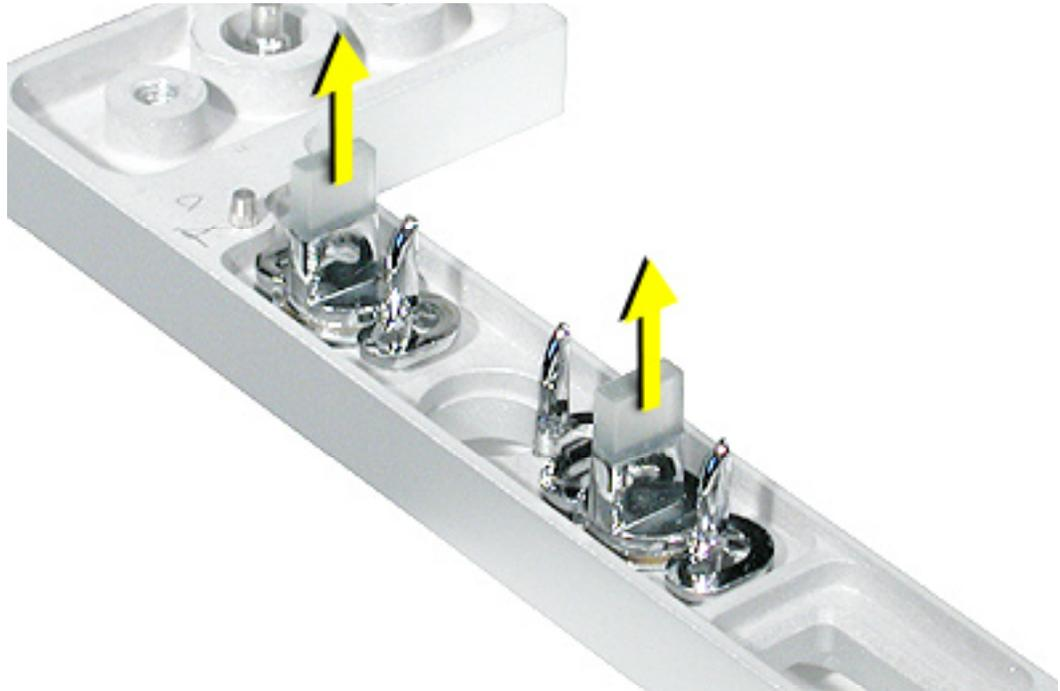
**Replacement Note:** Position the replacement buttons in the front bezel as illustrated.
