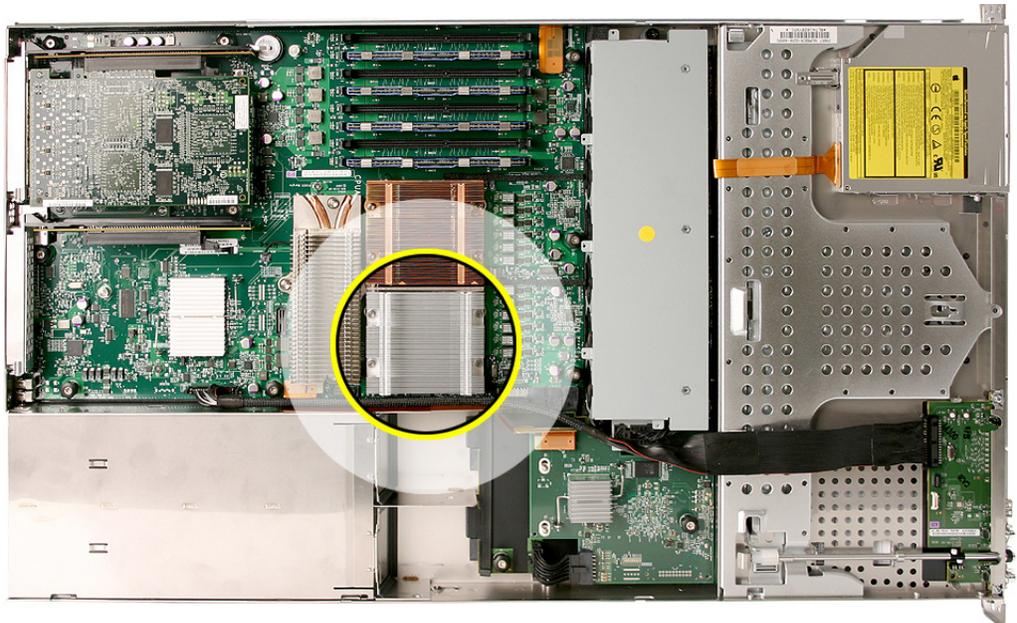
1. Loosen the four screws securing the heat sink that is closest to the DIMM slots (CPU A) in the order indicated below.
