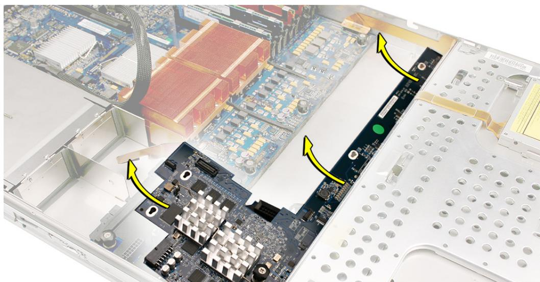
**Replacement Note:** When installing the Xserve RAID Card, lower the card into the enclosure at a slight angle (as shown), and carefully align the front edge of the card with the four alignment slots in the enclosure. Be careful not to let any Xserve RAID Card components come into contact with the standoffs or the enclosure as you install the card.
