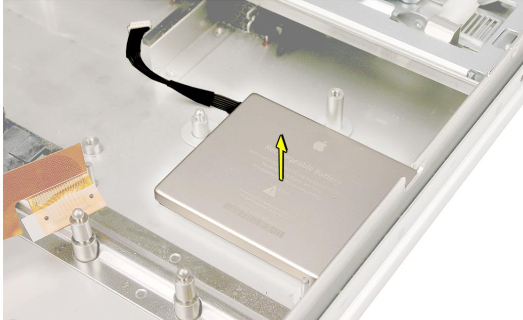
**Replacement Note:** Before installing a new battery, remove the protective film covering the adhesive on the underside of the battery. Then lower the battery into place on its three mounting posts.
