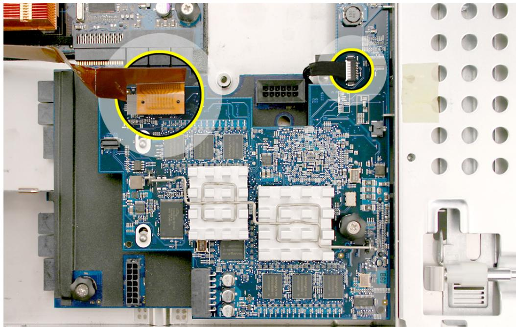
4. Release the thumbscrew that secures the Xserve RAID Card to the enclosure.
