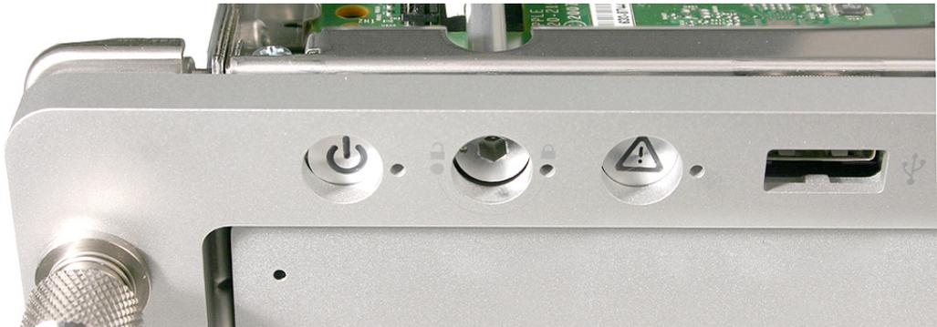
4. Replace the bezel brackets, four 4-mm long screws, and 8-mm long center screw with star washer.
