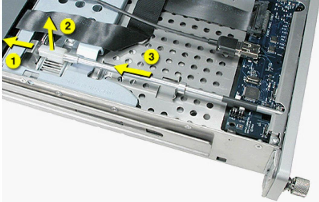
3. If you are replacing the plastic gear on the end of the rod, slide the gear off the rod.
