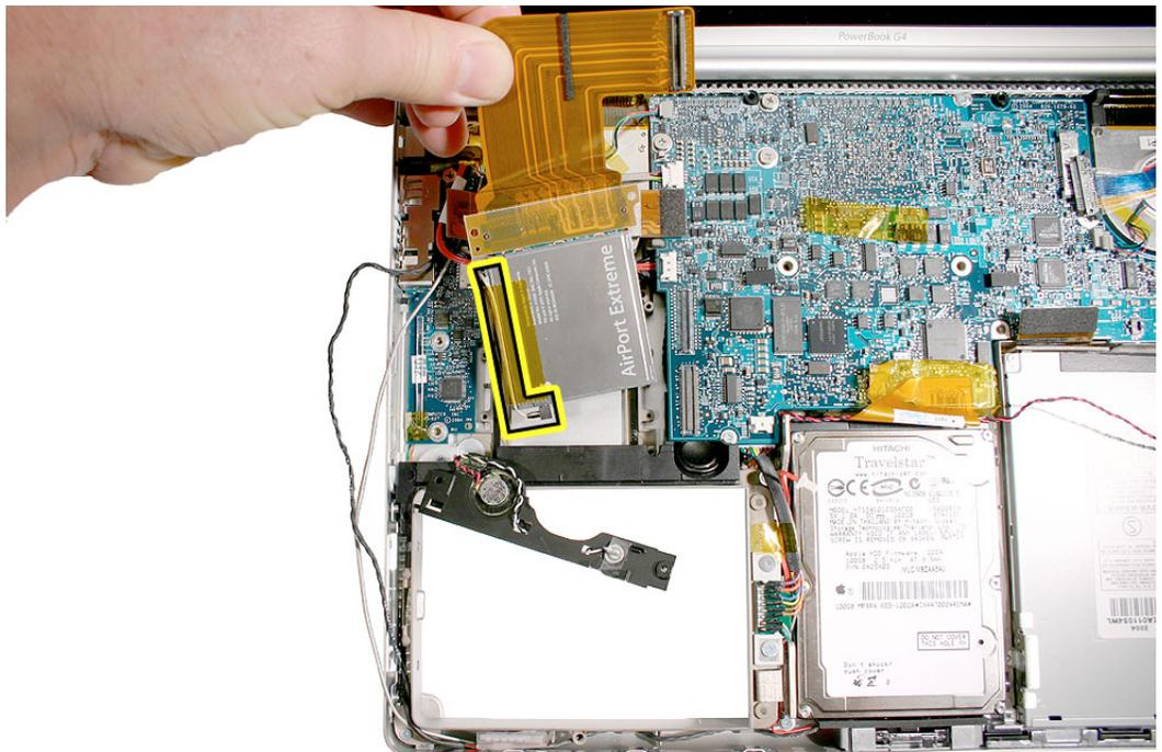
3. Firmly pull the antenna cable connector straight back from the card to disconnect it.
