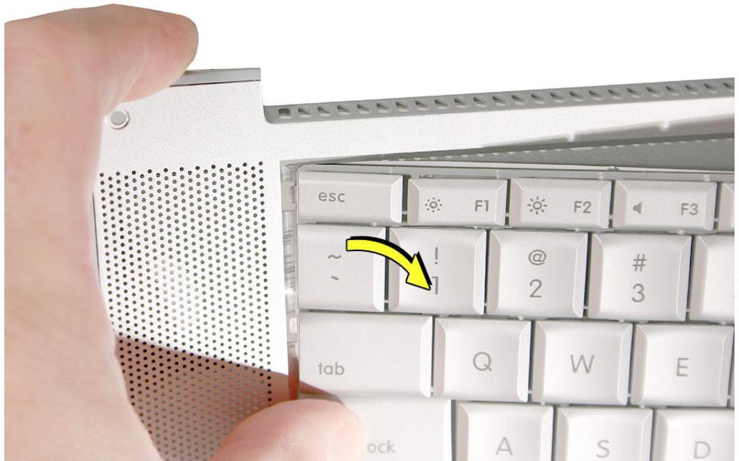
12. Lift the keyboard up to release the tabs along the bottom edge and carefully thread out the flex cables.
