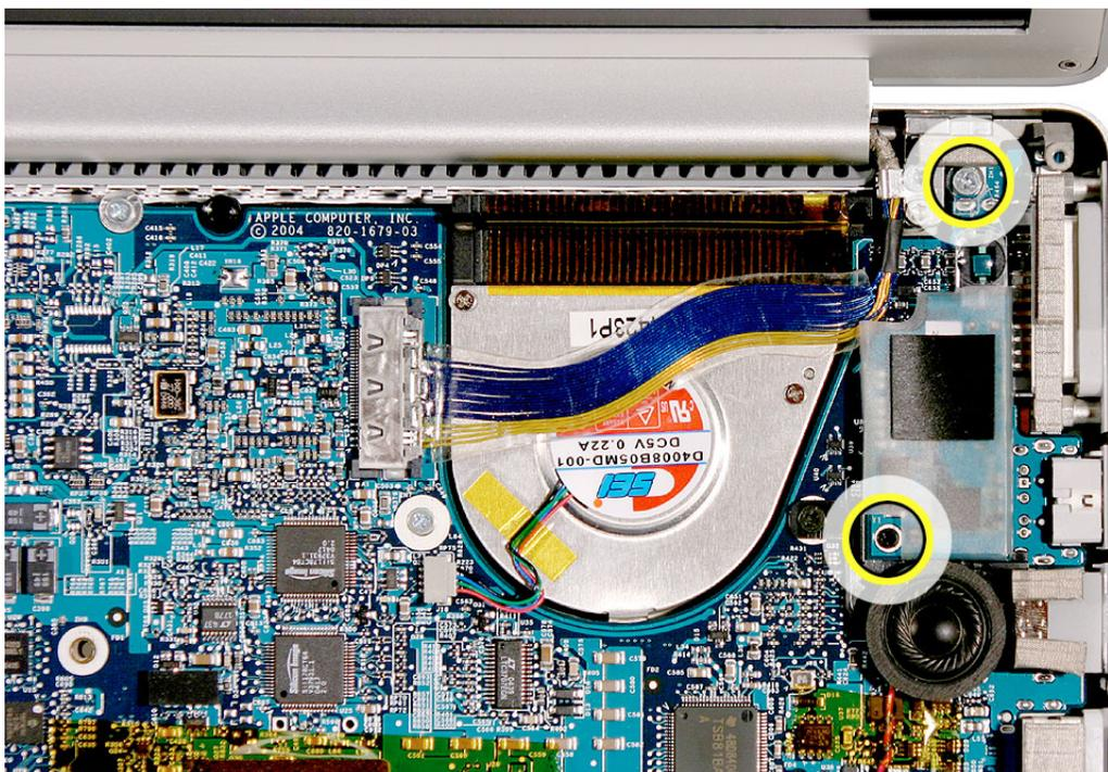
lift up on the board to disconnect it from the logic board (its connector is on the bottom of the board).
