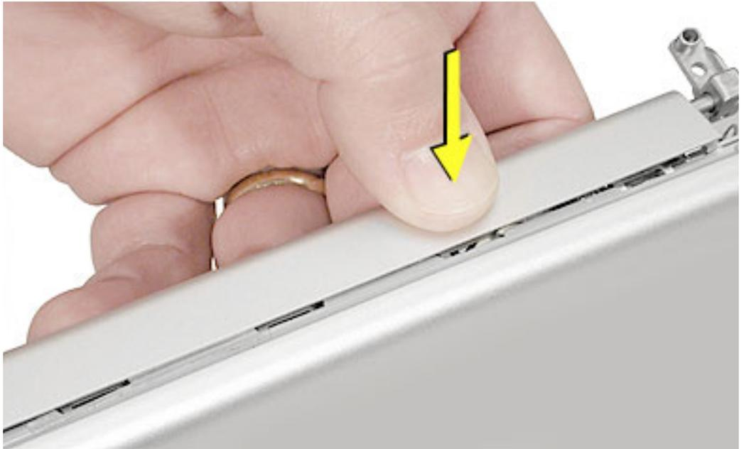
7. When the housing is loosened on sides and bottom, run a black stick along the gap at each bottom corner to slightly separate the rear housing from the display assembly.
