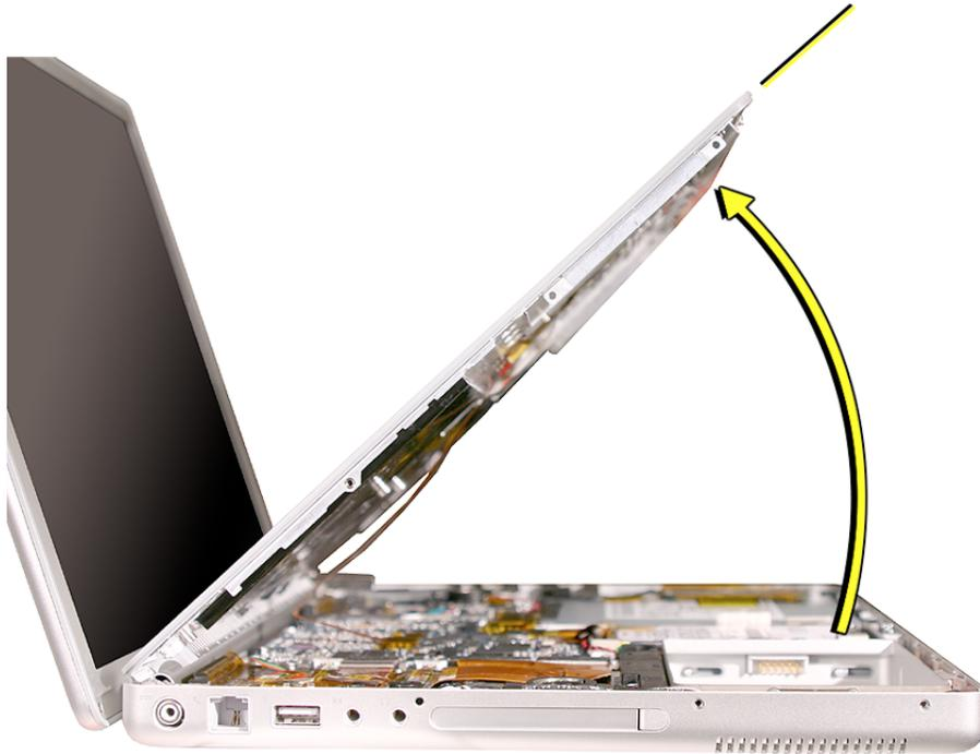
14. Remove any Kapton tape from the keyboard connector on the logic board, then use a black stick to disconnect the flex cable. Lift off the top case.
