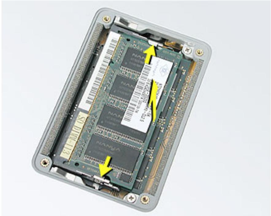
4. Pull the card straight back and out of the memory slot.
