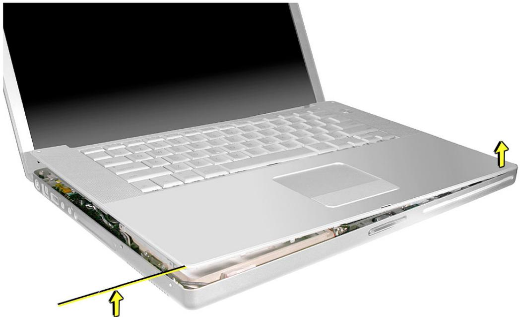
13. Lift the front of the top case and pivot along the back edge to about 45-degrees, to expose the keyboard flex cable connected to the logic board.
