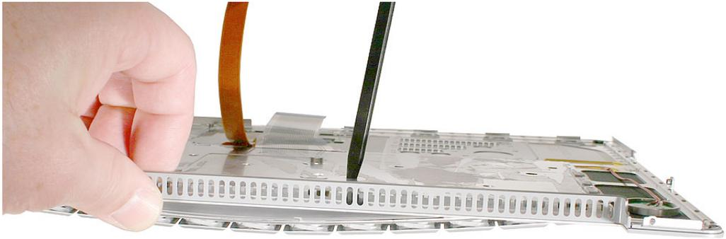
10. **Important:** During this procedure, do not allow the tabs or metal edge of the keyboard to scrape along the cosmetic surface of the top case, or damage can result.
