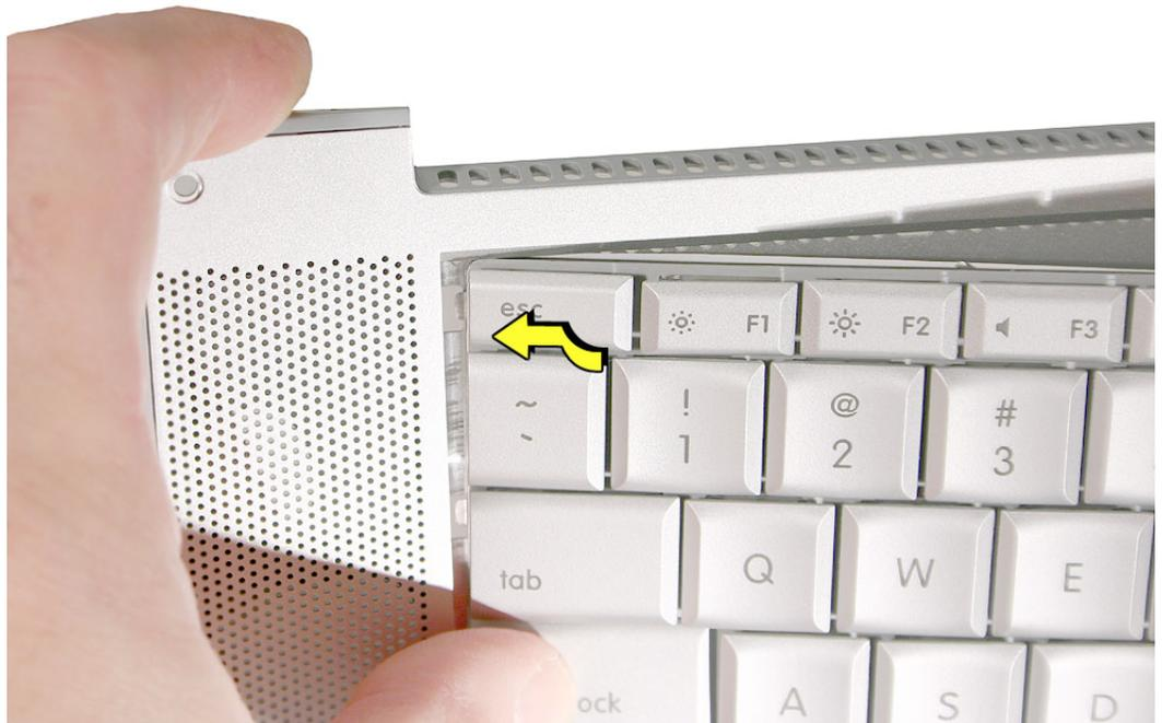
6. While supporting the keyboard in the top case, verify that the keyboard lays flat and that all the tabs have seated properly.
