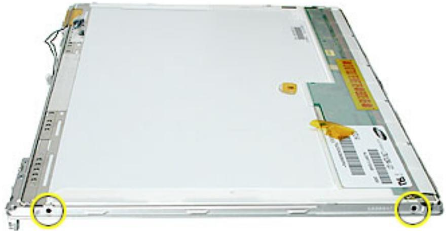
3. Remove the four screws at the top of the display.
