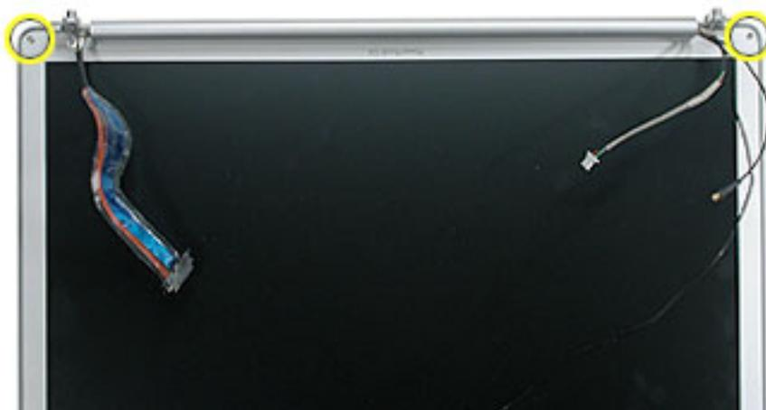
2. Holding the display assembly up on one side, carefully push with your thumbs on the edge bead to disengage the rear housing from three tabs on the side of the bezel.
