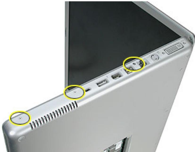
7. Open the computer slightly and rest it with the back facing up. Remove the two top screws along the back.
