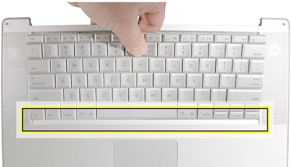
**Important:** During the next steps, do not allow the tabs or metal edge of the keyboard to scrape along the cosmetic surface of the top case, or damage can result.
