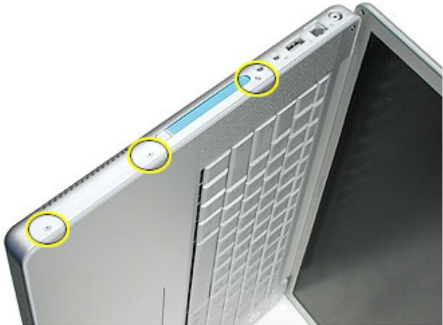
6. Turn over the computer and remove the three screws on the other side.
