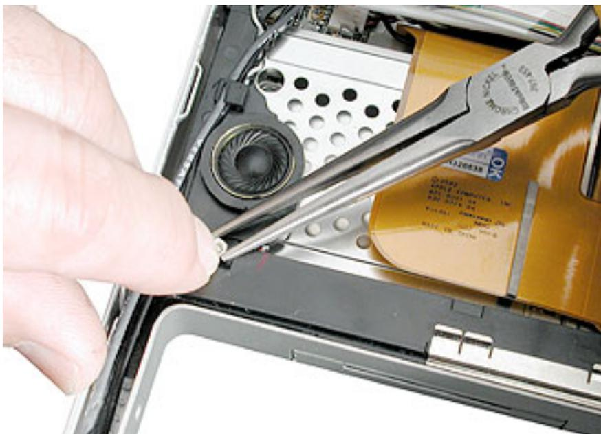
4. Install the replacement speakers, and reassemble the computer.
