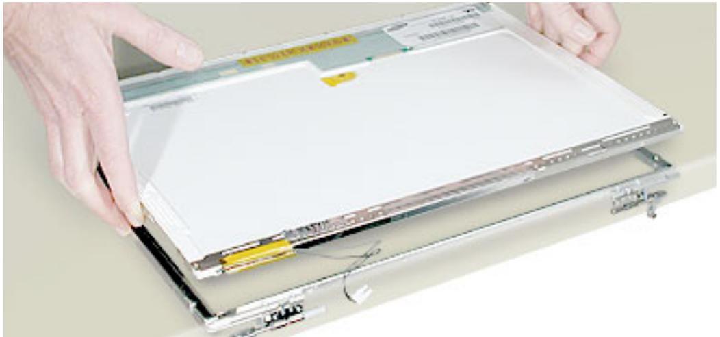
3. Lower the LCD panel and press its outside edges and the bezel into place.
