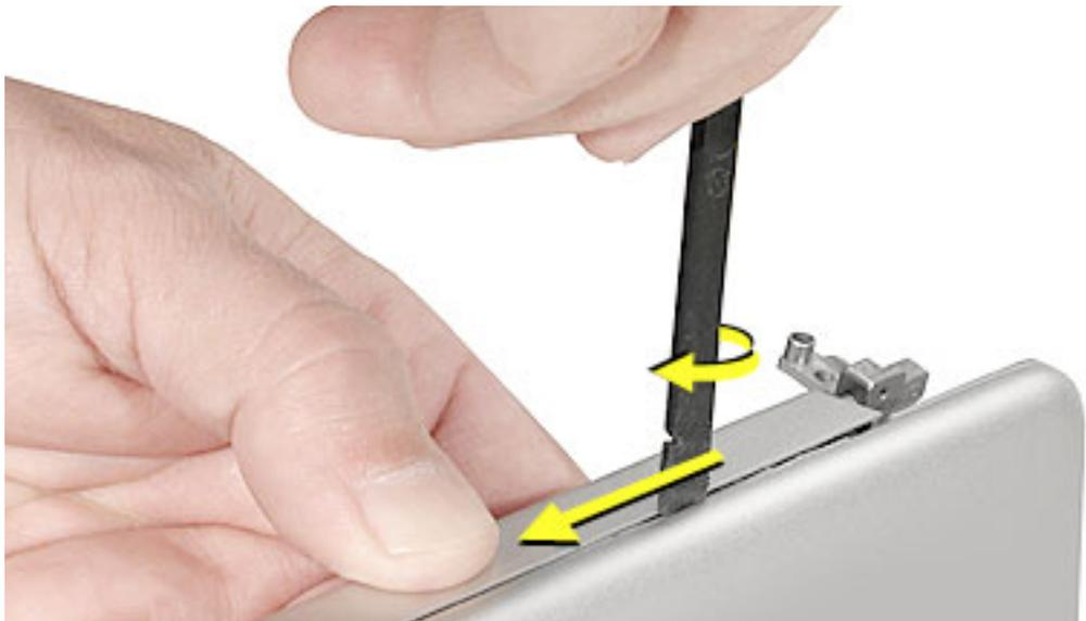
6. To help disengage the clips under the clutch cover, you may need to push down with your thumb over the clip location on the clutch cover, while slightly pulling the rear housing to disengage.
