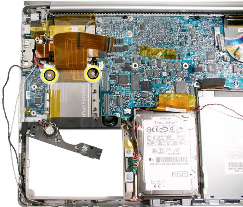
2. Slide out the AirPort Extreme card and flex cable assembly slightly, and peel up the Kapton tape to free the antenna cable from the card.
