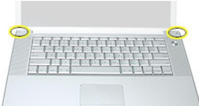
10. Along the left side, near the back, insert a black stick into the space between the top and bottom case. Work the black stick forward with a twisting motion until the black stick can be inserted on the left side of the front.
