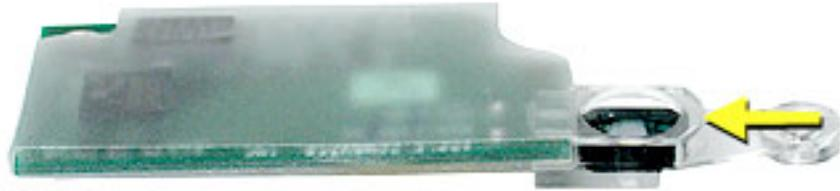
3. Press, where shown here, to secure the right ambient light sensor board connector to the logic board.
