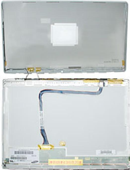
10. Note that the two antenna cables route along the side of the rear housing and are connected to the diversity board that is tucked into the channel of the clutch cover.
