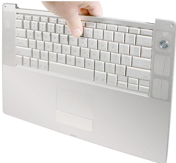
9. If needed, push through one of the top center keyboard screw holes, with the point of a black stick, to bow out the keyboard slightly.
