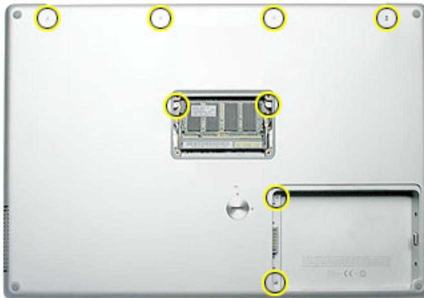
5. With the display open, rest the computer on one side. Remove the three screws.
