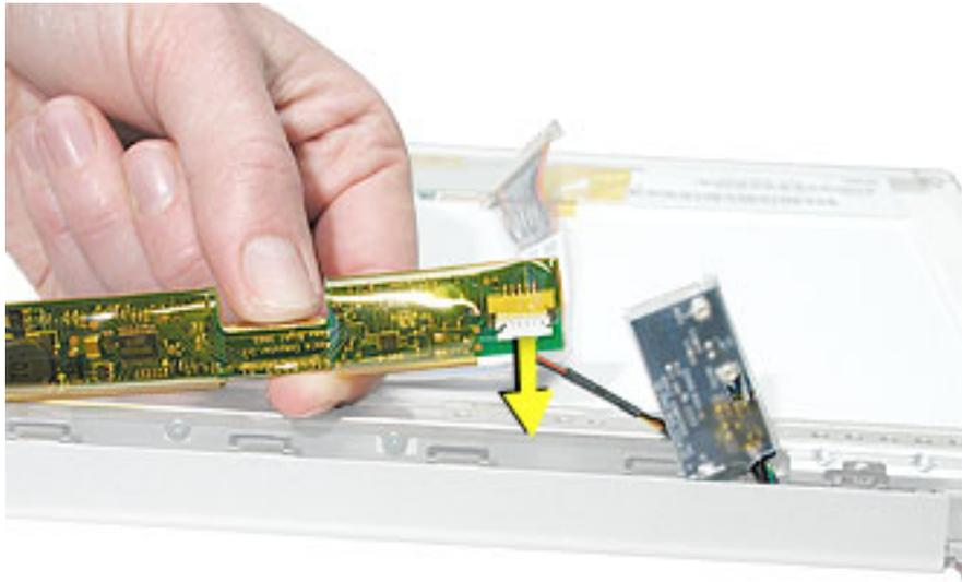
4. Tilt up the inverter board, and disconnect the cable at the left end of the board.
