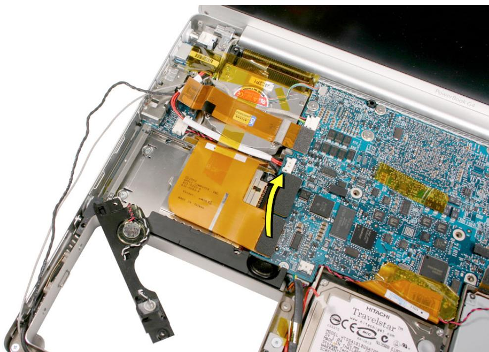
7. Disconnect the PC card cage flex connector, and remove the four screws.
