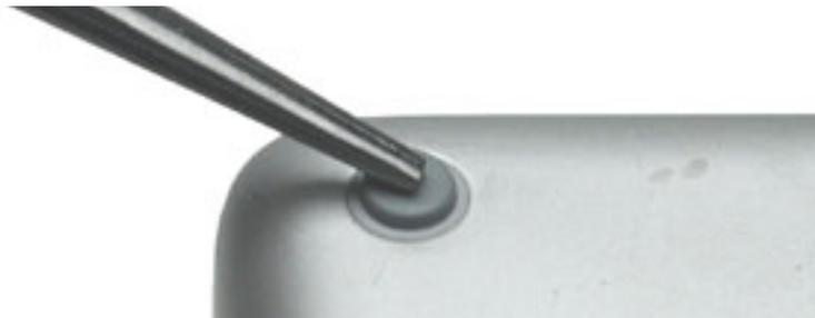
8. Before turning over the computer, allow the glue to set for at least 15 minutes.
