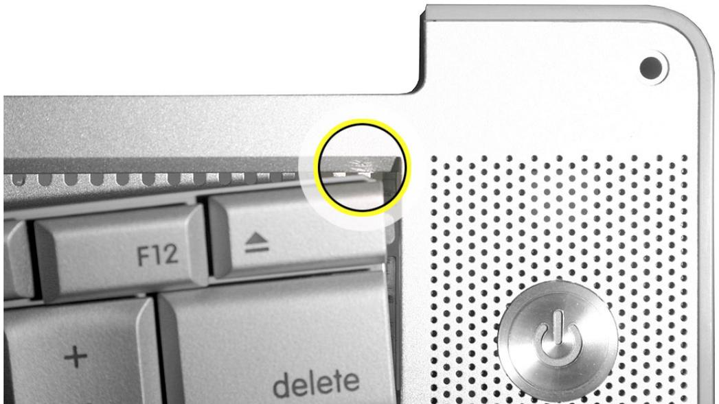
11. Use your finger to hold the bowed out keyboard. Continue to bow it out only enough for the tabs on one side of the keyboard to release cleanly. Repeat for the other side.
