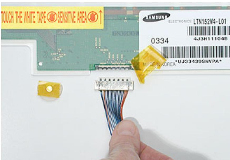
2. Peel up the metal tape securing the clutch end of the LVDS cable and reserve for reinstallation, or install new.
