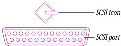
You can connect SCSI devices to the SCSI port in a chain-like fashion. The first device in the chain plugs into the SCSI port, the second device plugs into the first device, and so on.
