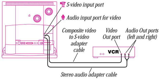
**Connection for input from a camcorder (composite connection)**
