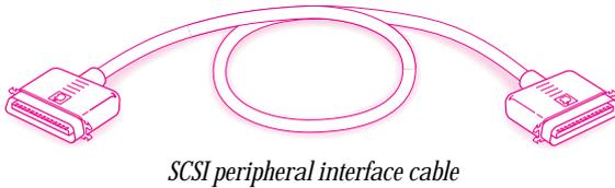
**Important** The total length of the cables in a SCSI chain should not exceed 6 meters (about 20 feet). For best results, use SCSI cables manufactured by Apple Computer.
