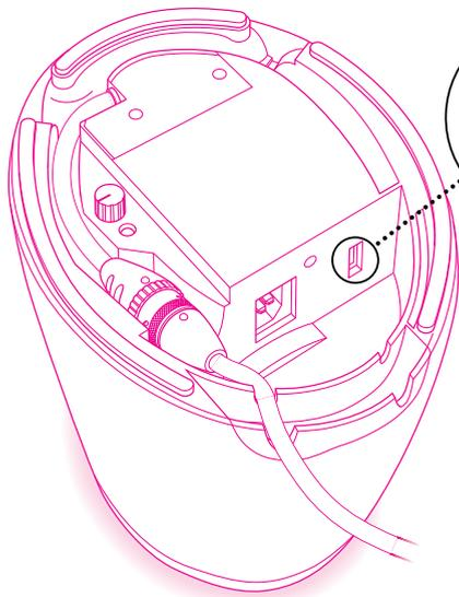
*Before you plug your computer in, check to see that the voltage switch in the bass unit is properly set. If you need to change the setting, insert a small screwdriver in the slot and slide the switch.*
