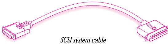
If the device is not the first one, use a SCSI peripheral interface cable to connect it to the last device in the chain:
