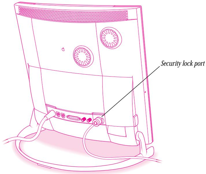
Follow the instructions supplied with the locking cable to secure it to your computer. When you install the locking cable, make sure the port cover plate is on.
