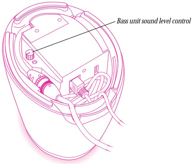
Once the bass unit level is set, the overall sound system volume is adjusted using the volume button on the front panel or the remote control.
