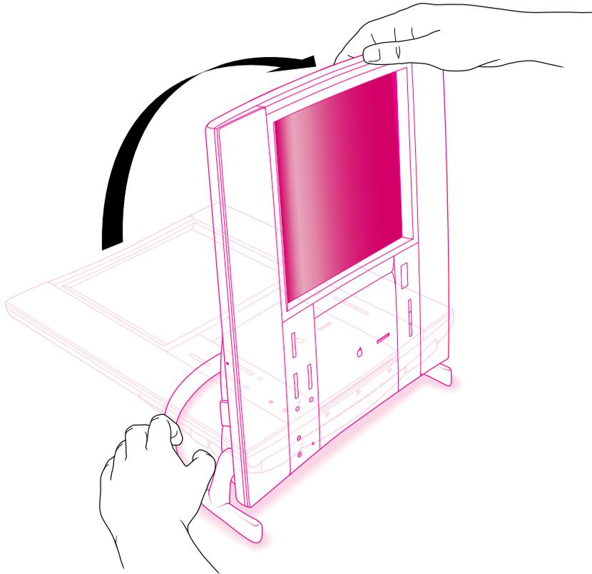
The screen should be vertical, tilted back by no more than a 15-degree angle, or tilted forward by no more than a 5-degree angle (to ensure that the CD-ROM drive operates correctly).
