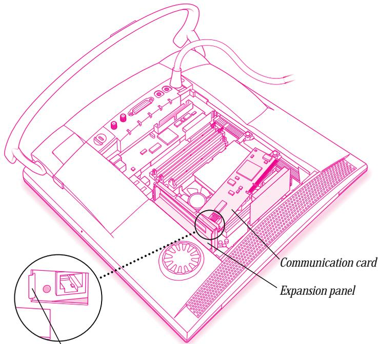
*If your communication card has a hook on it, be sure that the hook engages the expansion panel.*
