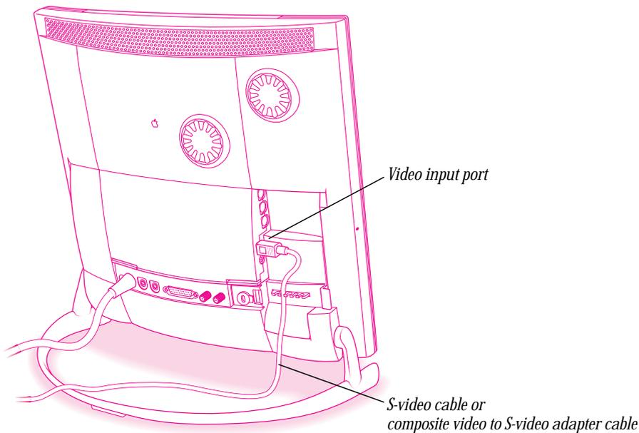
**Important** The S-video connector is a round plug with several small metal pins, which resembles other Macintosh connectors, such as those for a printer, modem, mouse, or keyboard. Don't confuse the connectors; they're not interchangeable.
