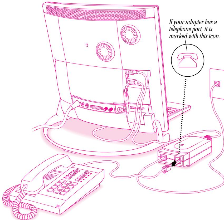
**Important** During lightning storms, disconnect your modem from the telephone jack to prevent possible damage to the modem.
