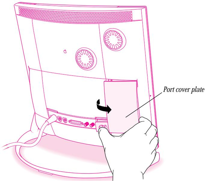
The port cover plate covers the ports for the modem (or GeoPort Telecom Adapter), keyboard, printer, and video equipment.
