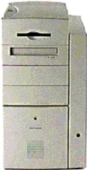
The Power Macintosh 8600 and 9600 Series computers share the same housing and feature a chassis design that allows you to access the logic board and its components (including the plug-in microprocessor card) simply by removing the side access panel. This flexible design makes the Power Macintosh 8600 and 9600 Series easier to service and upgrade.
