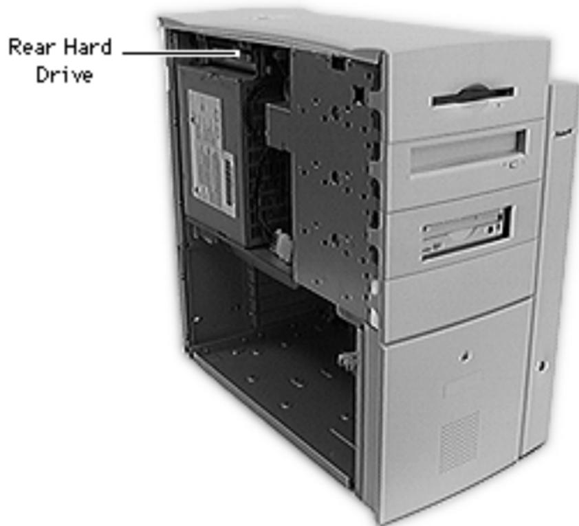
**Note:** This topic includes instructions for removing the rear drive carrier and rear hard drive.
