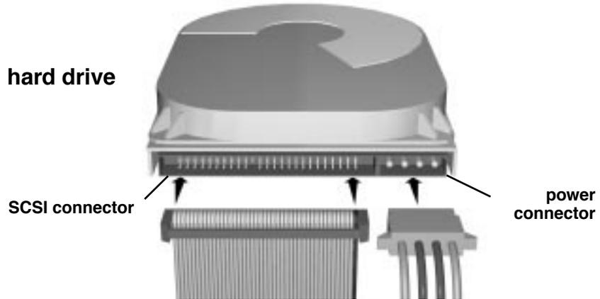
8. Find an unused four-pin power cable in the set of cables coming from the power supply (the power supply is in the right rear of the computer, on the bottom) and connect that cable to the rear of the drive, being careful to match the beveled corners of the plug to those of the socket.
