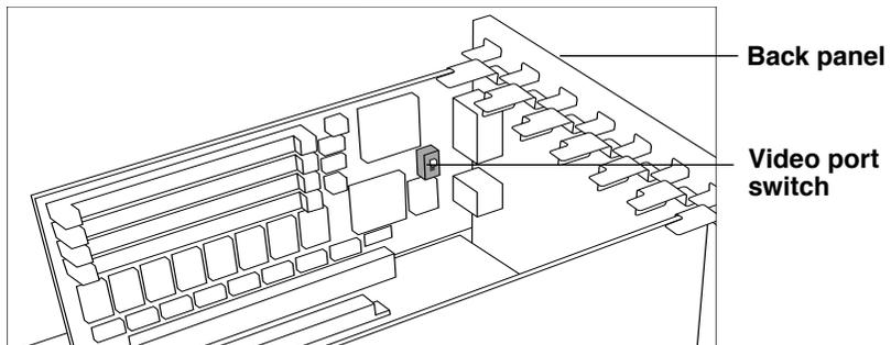
3. Flip the switch to the up position to enable the Macintosh-standard port. Flip it down to enable the VGA port.
