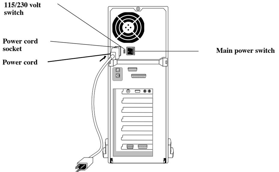
**WARNING!** For your safety, the computer is equipped with a three-prong plug designed to be used with a grounded electrical outlet. If you do not have access to an appropriate outlet, have an electrician install one. Do not use your computer with a three-prong adapter in an ungrounded outlet.
