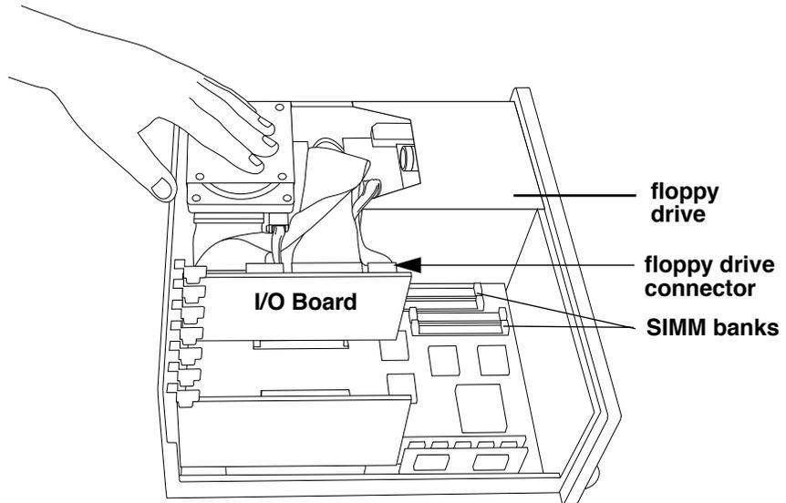
3. Disconnect the floppy disk drive connector, the CD audio connector, if you have one, (below the floppy connector), and the speaker connector (below the CD audio connector) from the I/O board and move those cords out of the way.
