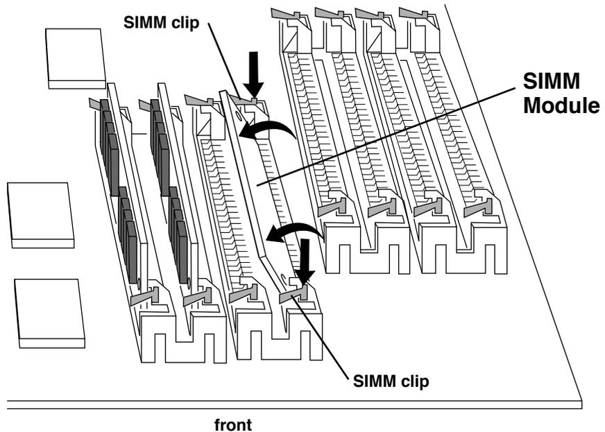
1. If you need to remove a SIMM module to make room for a higher-capacity one, reach in and push down and out on the tiny handles which stick up from the small metal SIMM clips at each end of the SIMM slot.
