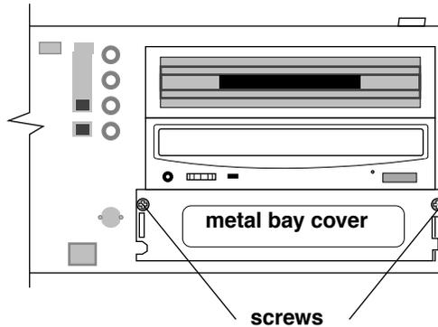
**Note:** The slot under the floppy drive on the desktop model and the top slot on the tower drive may have a metal plate without screws, which is attached by two thin strips of metal. To remove *that* type of plate, simply bend it back and forth several times until it comes loose, and remove it.
