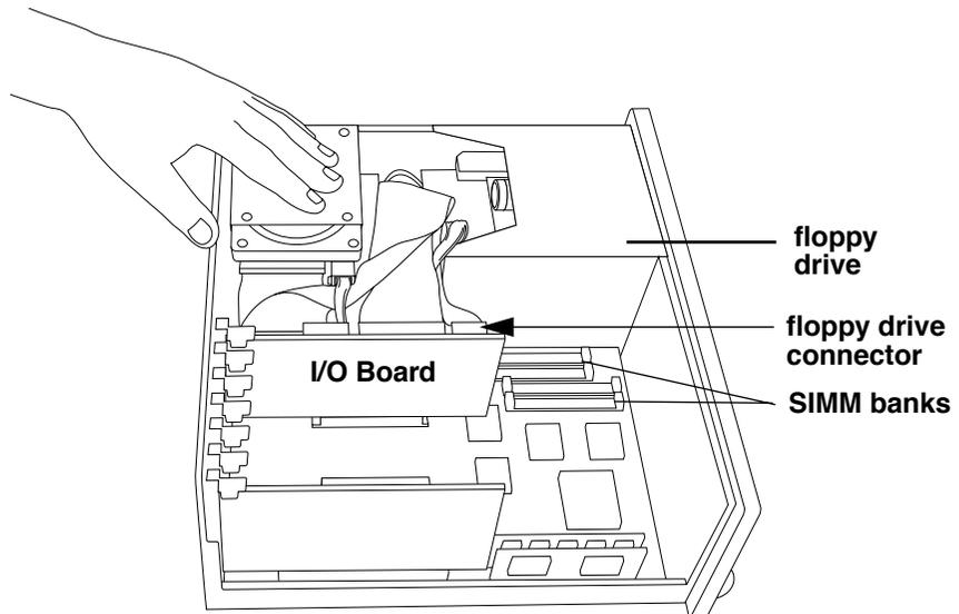
3. Disconnect the speaker connector, which is on the I/O board below the floppy disk drive connector.
