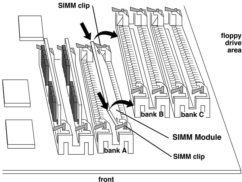
1. To insert a SIMM module, hold the module by the ends with the contacts down and the slotted end toward the back of the computer.
