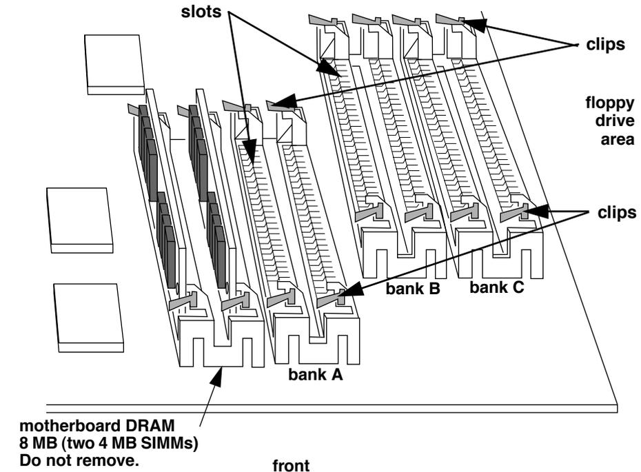
The motherboard bank is the pair of clips farthest from the floppy drive cavity, A is next, etc. The motherboard bank comes with two 4 megabyte SIMMs, which are required for the system to work. Do not replace the SIMMs in the motherboard bank with SIMMs of any other capacity; that bank will only work with two 4 megabyte chips.
