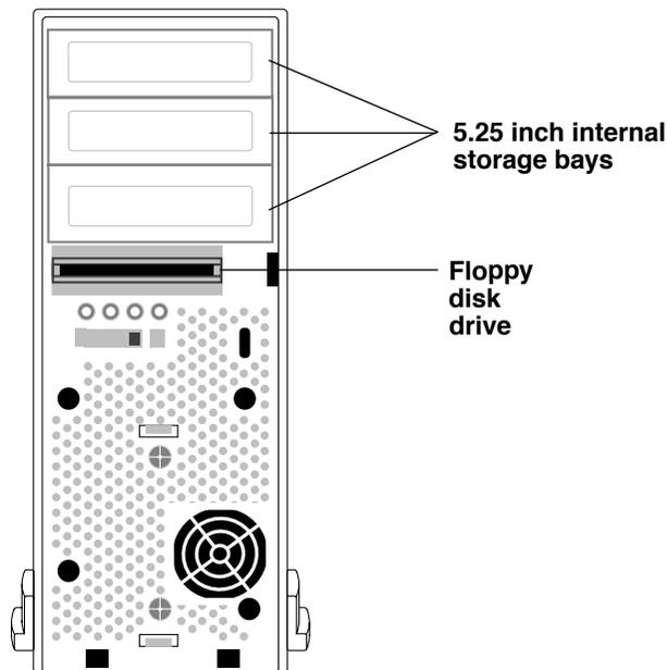
Rails for mounting internal devices are available from Power Computing for a nominal fee; contact our Sales Department at 1-800-999-7279. Rails, as well as adapter trays for installing 3.5 inch drives in the 5.25 inch bays are also available at most computer parts stores.
