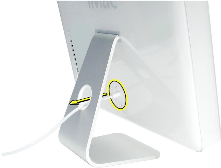
3. Place a soft, clean towel or cloth on the desk or surface. Hold the sides of the computer and slowly lay the computer face down as shown.
