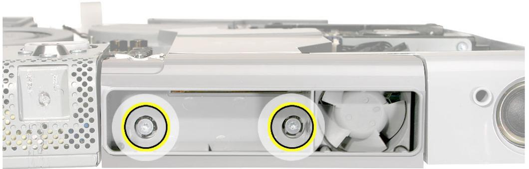
2. Turn over the computer assembly and route the fan cable through its cable guides. Connect the fan cable to the connector on the logic board.
