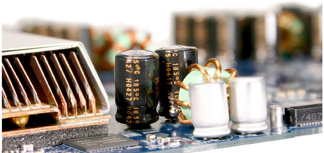
6. If the logic board has bulged or vented capacitors, replace the logic board.
