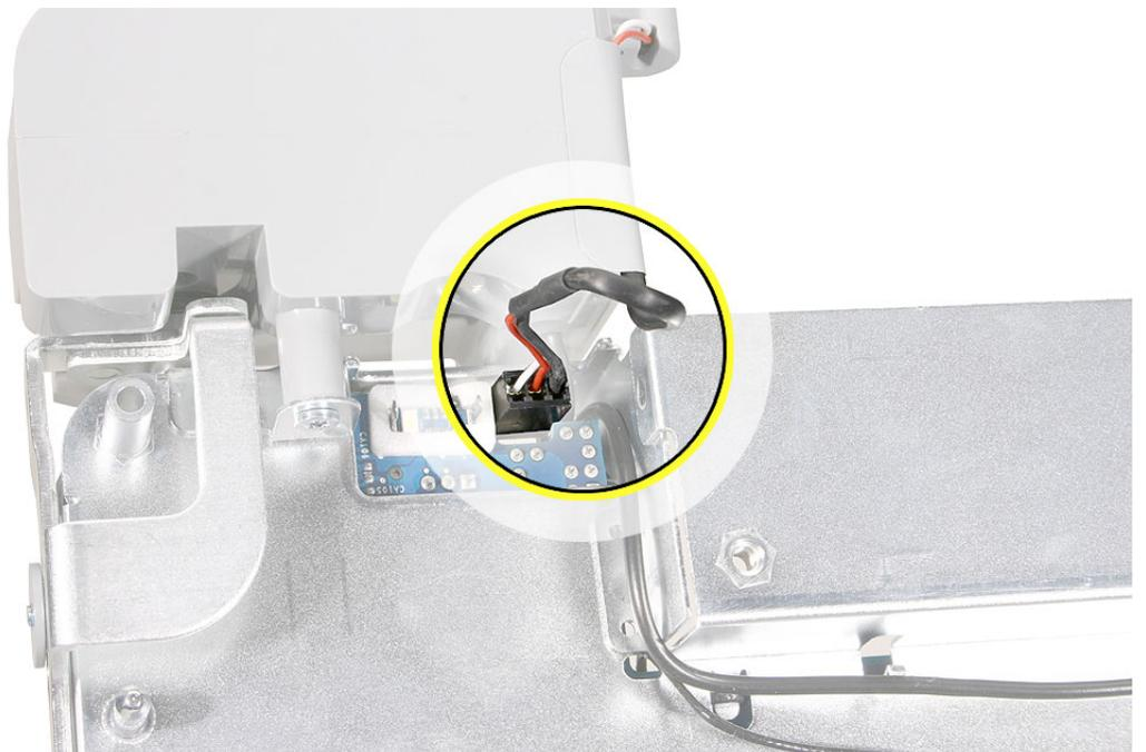
6. Route the widest speaker cable connector through the midplane chassis opening.
