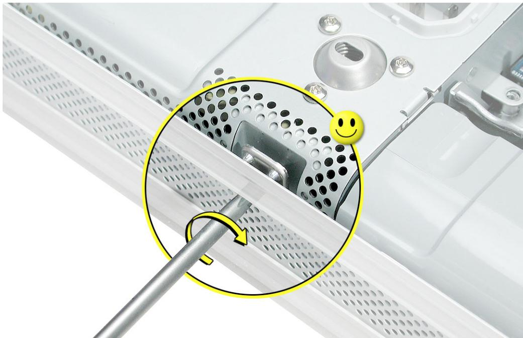
29. Lift up the power supply at the sides approximately five mm or until it touches the middle case screw.
