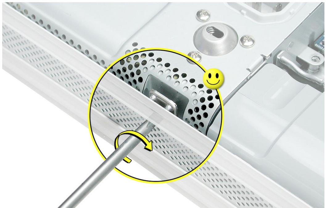
16. Remove the six screws (four identical, short, brass-colored screws in the channel along the top, and two screws on the left side of the board).
