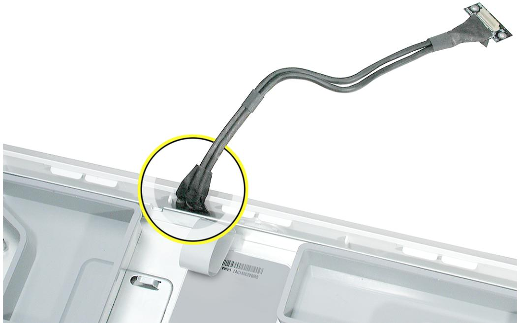
36. Locate the pull tab. Pull the tab up to release the midplane assembly from the display/bezel assembly.
