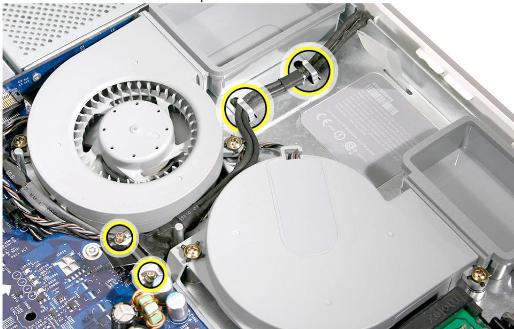
6. Replace the fan duct and replace the two screws.
