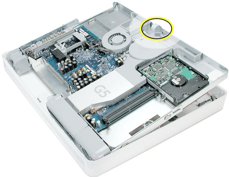
22. Push the inverter cables down through the openings on the midplane assembly. Lift the midplane assembly up and set it aside. **Important:** Return this midplane to Apple in the packaging provided
