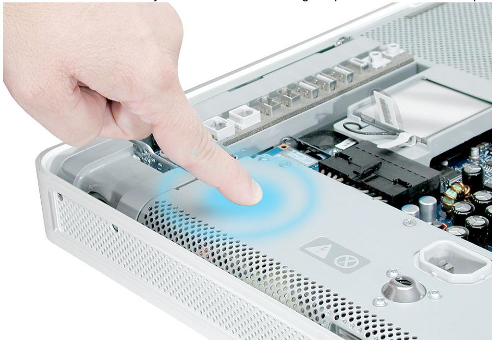
3. Locate the AirPort Extreme card. The battery is located below the AirPort Extreme card. **Note:** If an AirPort Extreme card is not installed, go on to step 7.
