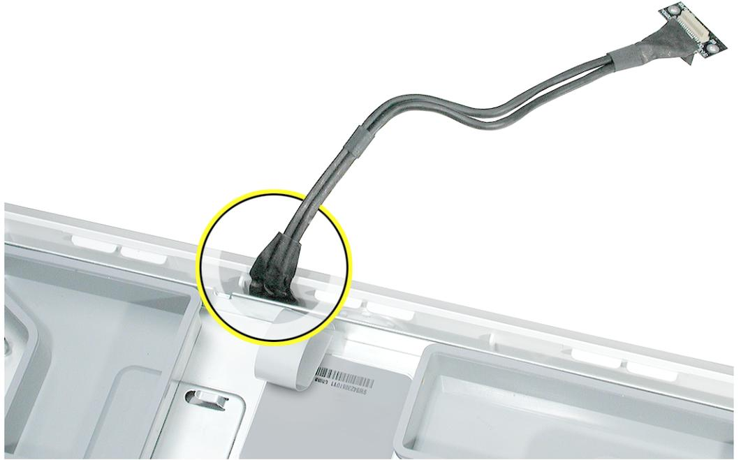
21. Locate the pull tab. Pull the tab up to raise the midplane assembly. Then hold the midplane on each side and pull the midplane up and out of the display/bezel. If it is difficult to remove, make sure the captive power supply screw was turned completely counterclockwise. **Note:** The captive screw sleeves (near the speakers) on the midplane fit tightly into the display/bezel assembly, tug the midplane to release it.
