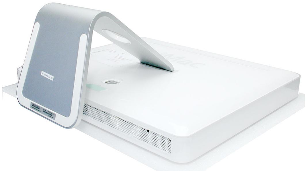
4. Locate the three case screws circled below. You may have to lift the metal foot to locate the middle case screw. **Note:** These screws are captive; they are part of the display/bezel assembly and cannot be removed.
