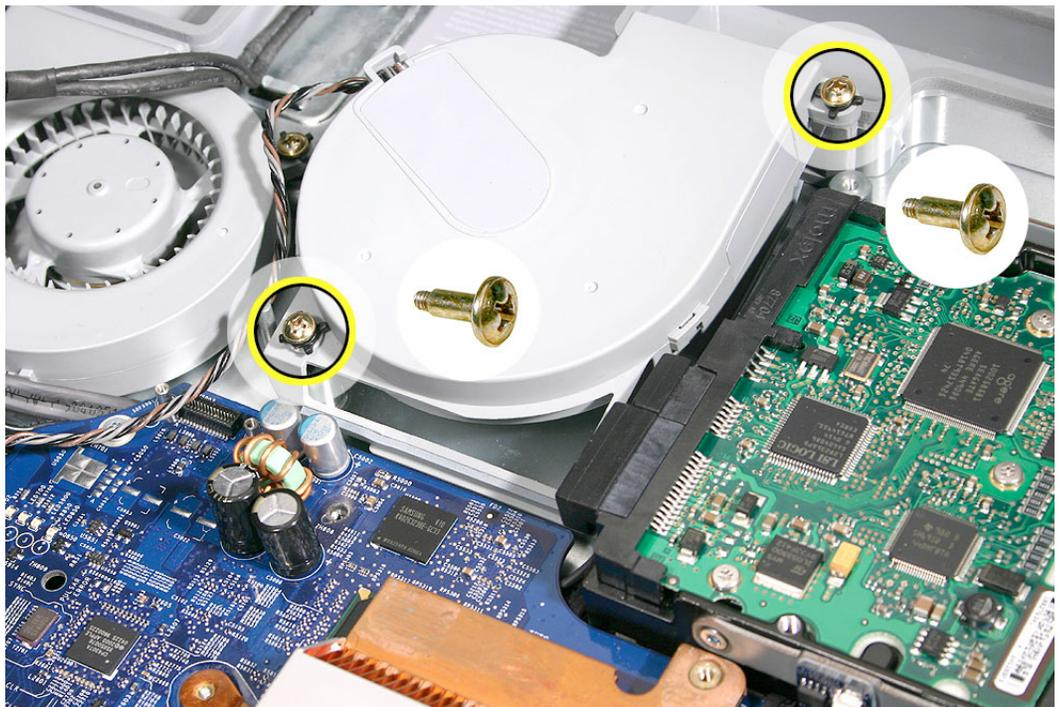
5. Replace the two screws connecting the video cable to the logic board and place the video cable under the metal clips.
