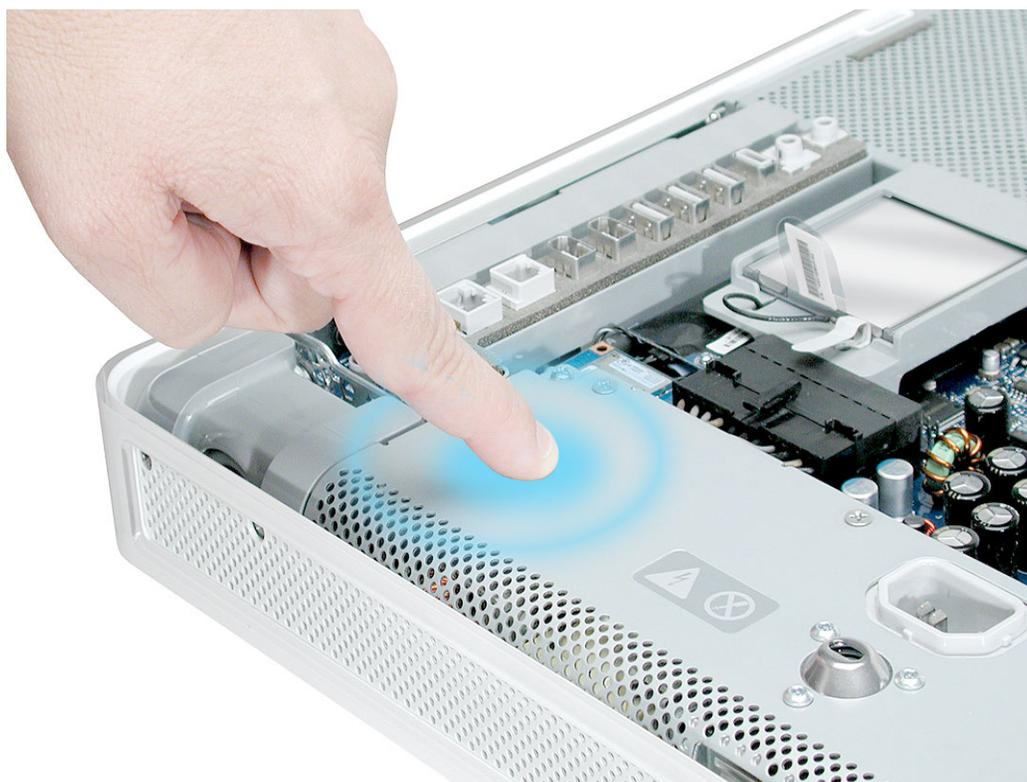
3. Locate the hard drive near the top right corner.
