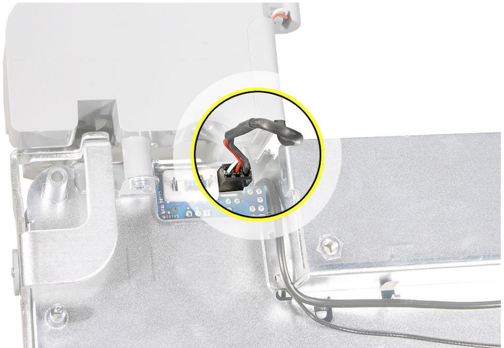
5. Note the routing of the microphone cable. Peel up the speaker tape, and lift up the microphone cable from the speaker channel.
