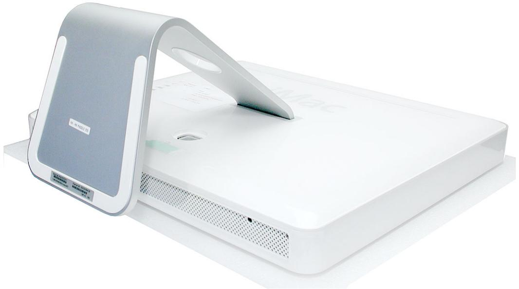
4. Raise the foot and use a Phillips #1 screwdriver to loosen the three screws at the bottom of the computer by turning them completely counterclockwise. These are “captive screws,” which means they're not supposed to come all the way out.
