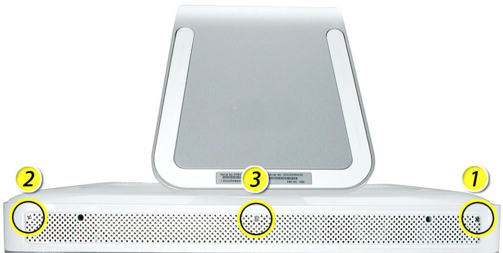
5. As you hold the metal foot, tilt the back cover up and lift it away from the computer. The back cover with the foot attached should come off easily. If it doesn't, make sure the screws are turned completely counter-clockwise, but not too far.
