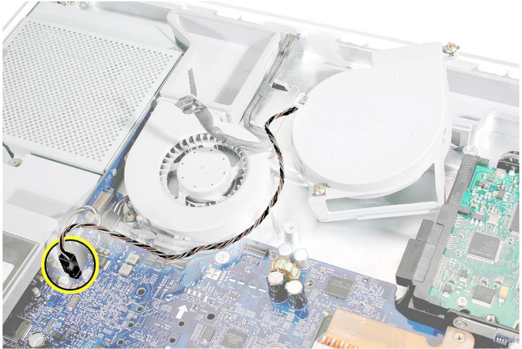
4. Place the two screws into the grommets on the fan. Lower the fan into the computer, making sure the bottom end of the fan tucks under the logic board. Tighten the two fans screws.
